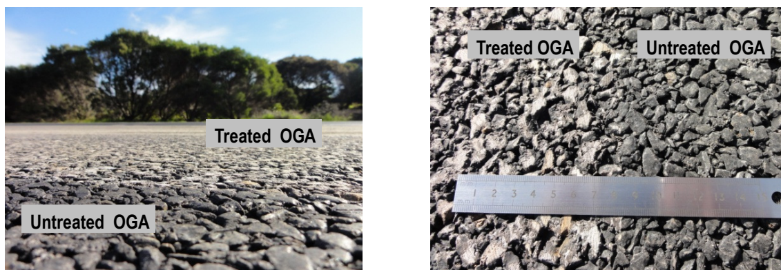
Figure 2 –OGA Treated by shaving on Section 2.
