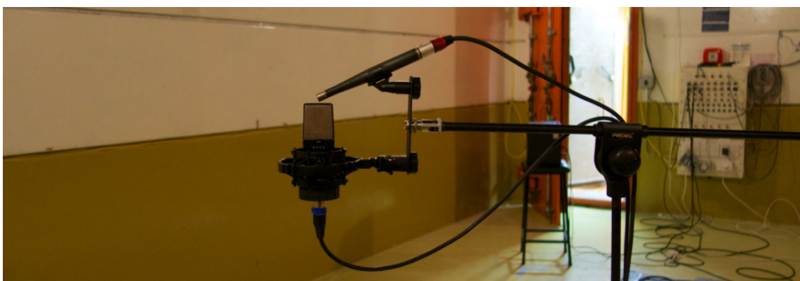
Figure 4 – The first microphone arrangement for “System 2”: a Brüel & Kjær Type 4007 pressure microphone (top) with an AKG C414 B-ULS microphone set to a figure-of-8 pattern (bottom). This is setup in a reverberation chamber at The University of Auckland for a calibration measurement.
