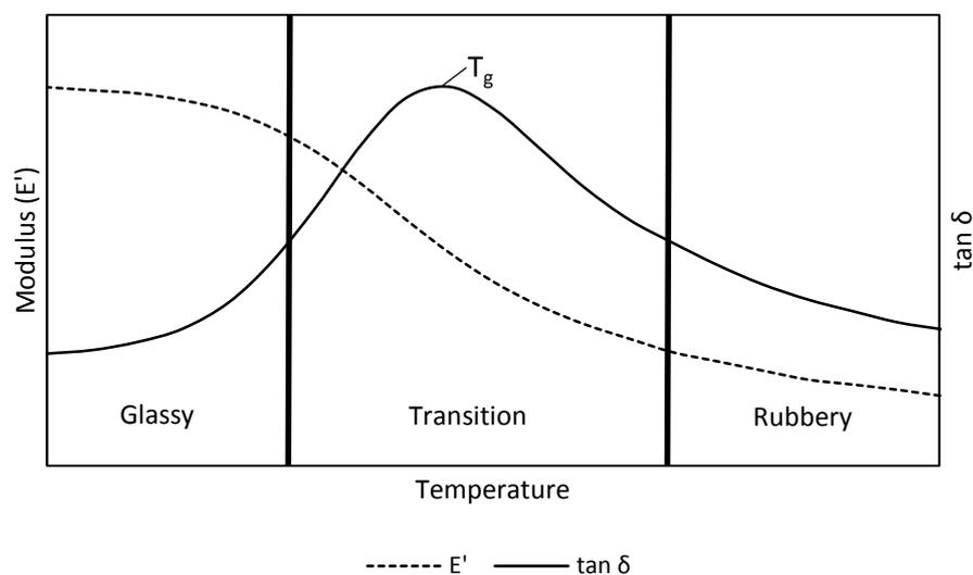
Figure 1 – Damping ( $\tan \delta$ ) and modulus ( $E'$ ) as a function of temperature with the three regions marked
