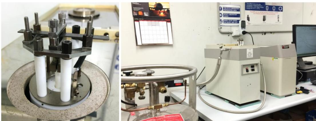
Figure 2 & 3 – The DMA test chamber and system during the calibration process
