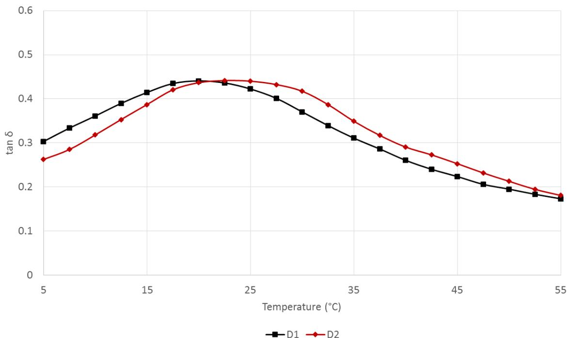
Figure 7 – DMA results for viscoelastic materials with different sample processing methods
