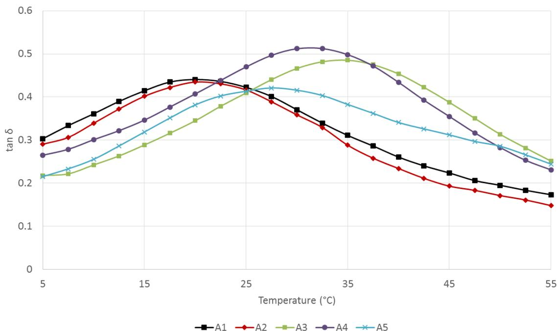
Figure 4 – DMA results for viscoelastic materials with different fillers
