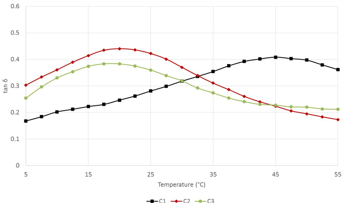
Figure 6 – DMA results for viscoelastic materials with different plasticiser content
