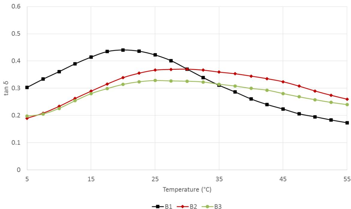
Figure 5 – DMA results for viscoelastic materials with different polymer content
