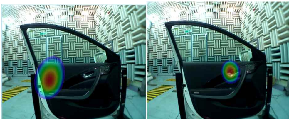
Figure 8 – Results of sound field visualization of door latch operating moment
