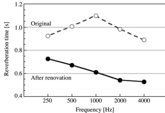
Figure 5 – Comparison of mean reverberation times between original (dotted line) and after the renovation (solid line).
