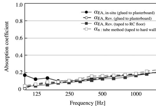
Figure 7 – Comparison of absorption coefficients of RWB measured by EA-method (in-situ), EA-method (glued to plasterboard, in Reverberation room), EA-method (double-face taped to RC floor, in Reverberation room) and tube method.
