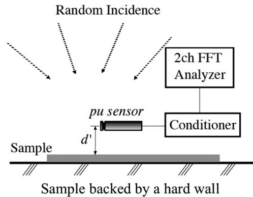
Figure 3 – EA-method measurement setting.
