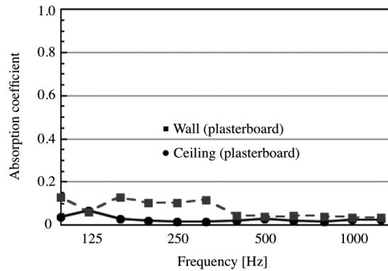
Figure 6 – Absorption coefficients of wall and ceiling measured in-situ by EA-method.
