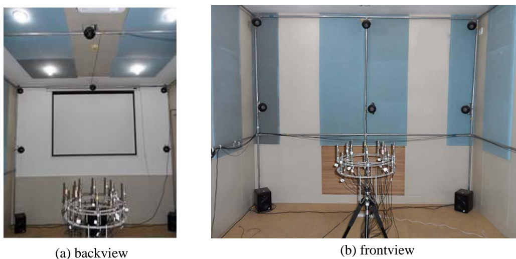
Figure 3 – Arrangement of loudspeakers and microphones
