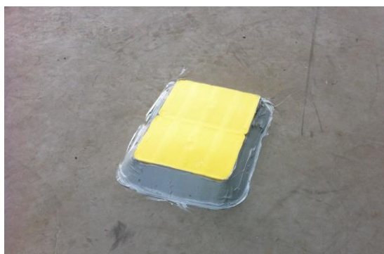
Figure 3 Typical packing under jack-up mounts.
