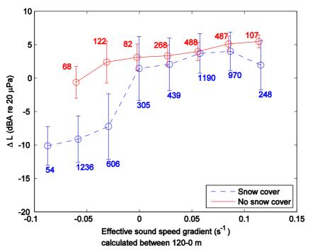
Figure 3 - Relative SPL (ΔL) (calculated with eq. 2) versus sound speed gradient during different ground conditions for the Dragaliden site. The sound speed gradient is calculated from 120 m height to the ground. The numbers indicate the total number of selected measurements within each bin and the circles (o) gives the median in each bin. The bars indicate one standard deviation of the data.
