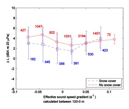
Figure 4 - Relative SPL ( $\Delta$ L) (calculated with eq. 2) versus sound speed gradient during different ground conditions for the Ryningsnäs site. The sound speed gradient is calculated between 120 m height and the ground. The numbers indicate the total number of selected measurements within each bin and the circles (o) gives the median in each bin. The bars indicate one standard deviation of the data.
