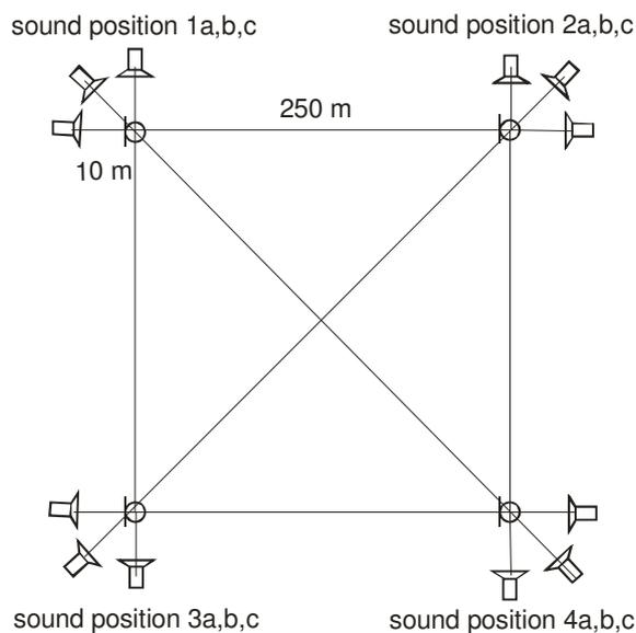
Figure 1 – The test setup with the source and receiver positions
