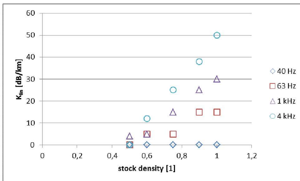
Figure 2 – attenuation coefficients for the reduced pine forest stand
