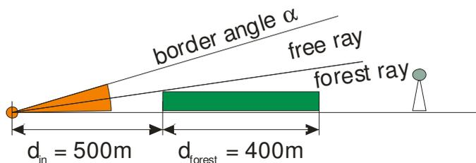
Figure 6 – The two sectors of the relevant sound energy from a source on one side of a forest to an immission point on the other side
