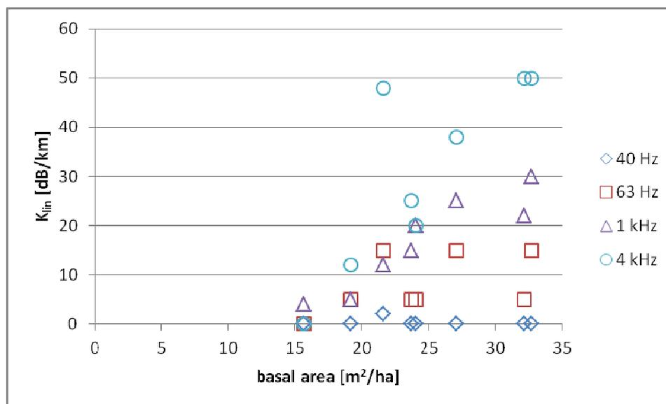
Figure 3 – attenuation coefficients for pine forest stands no. 2 and no.3 and for the oak tree plotted against basal areas
