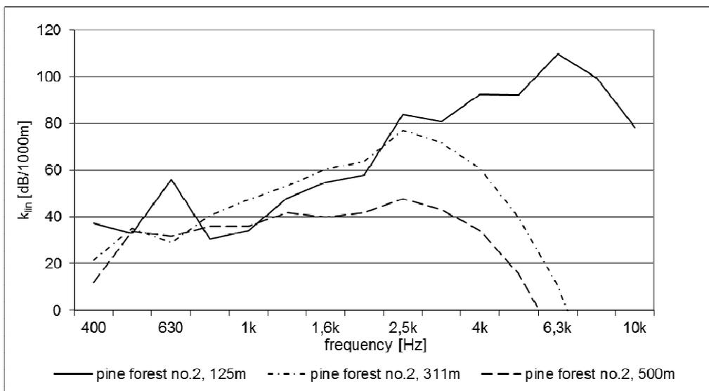
Figure 5 – attenuation coefficient for pine forest no. 2 plotted against frequency
