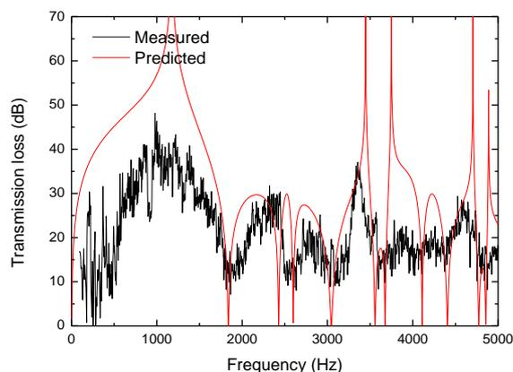
Figure 6 - Comparison between measurement and prediction
