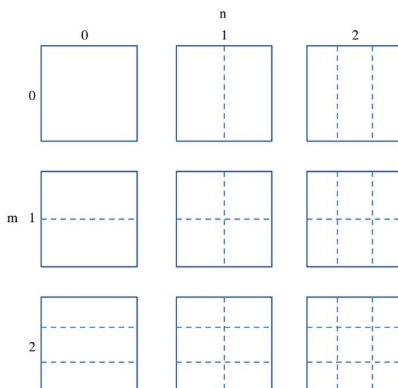
Figure 2 - Nodal lines for transverse pressure distribution in a rectangular duct
