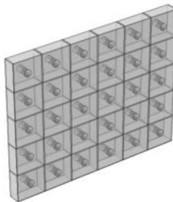
Figure 5 - A noise barriers using rectangular chambers
