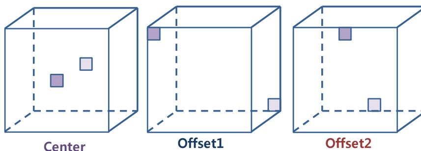
Figure 3 - Three types of rectangular chambers used to verify effects of inlet/outlet position
