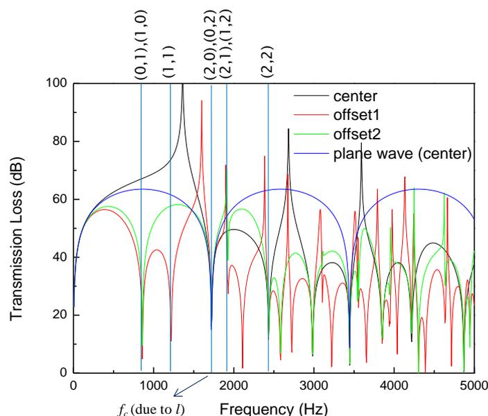
Figure 4 - Transmission loss of three types of rectangular chambers
