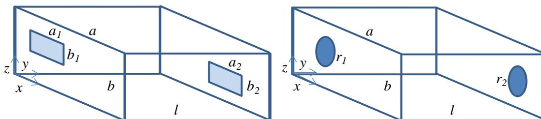
Figure 1 - Through-flow type rectangular chambers.
