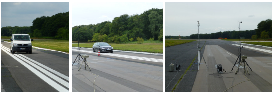
Figure 2 – Coast-By measurements. Left: Measurement with minibus. Middle: Measurement with passenger car. Right: Microphones, speed indicator and devices for meteorological measurements.
