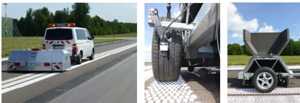
Figure 3 – Left: Enclosed CPX trailer with towing vehicle. Middle: SRTT with microphones on mandatory positions. Right: Open trailer box with SRTT.
