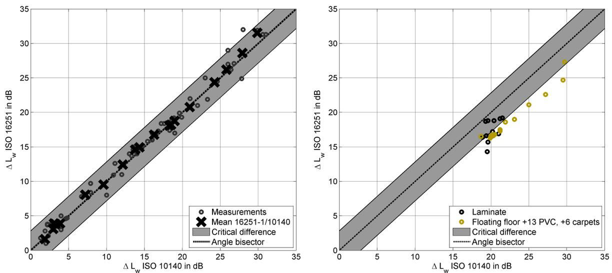
(a) Comparison between the weighted impact sound reduction  $\Delta L_w$  obtained at three different compact measurement setups according to ISO 16251 (2) and three different test facilities according to ISO 10140 (1).
