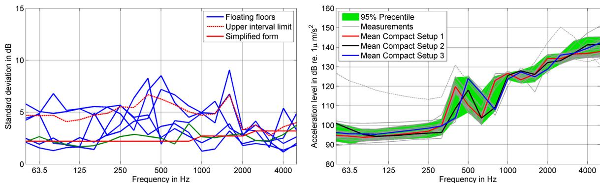
(a) Standard deviation of the differences of the acceleration levels for every position of the accelerometers for measurements on six screeds.
