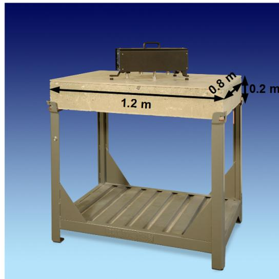
Figure 1 – Compact measurement setup for heavyweight floors.
