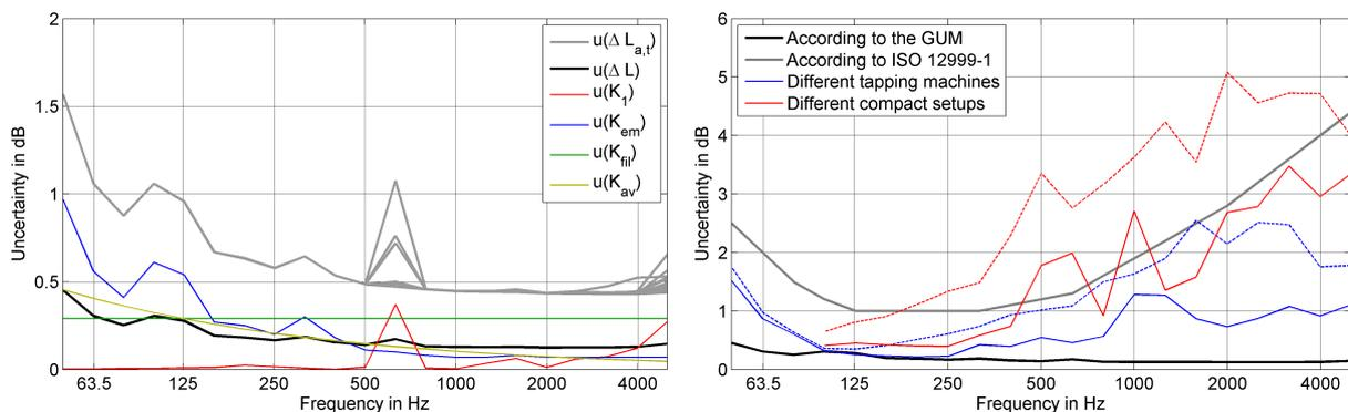
(a) Single components of the uncertainty for measurements at the compact measurement setup.
