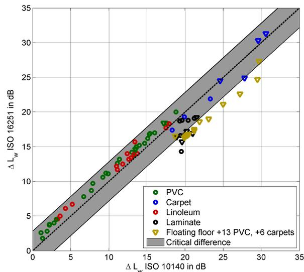
Figure 6 – Comparison between the weighted impact sound reduction  $\Delta L_w$  obtained according to ISO 10140 (1) and ISO 16251 (2) with perspective to the introduced validation procedure based on the standard deviation of the acceleration level differences. Invalid classified measurements are marked as triangles.
