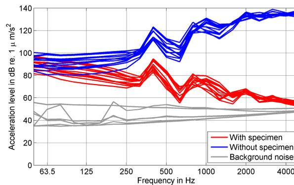
Figure 7 – Acceleration levels with and without a specimen and background noise level.
