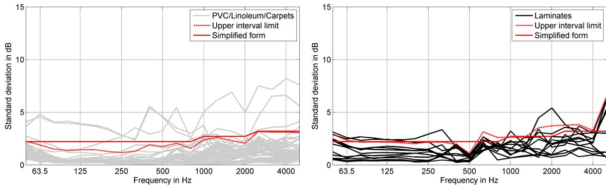
(a) Standard deviation of the differences of the acceleration levels for every position of the accelerometers for measurements with 52 soft floor coverings like linoleum, PVC and carpets.
