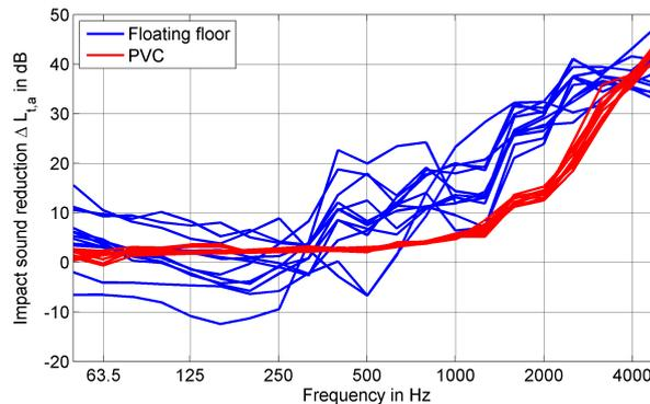
Figure 3 – Difference of the acceleration levels for every position of the accelerometers for measurements with a screed (blue) and with a PVC (red) covering.
