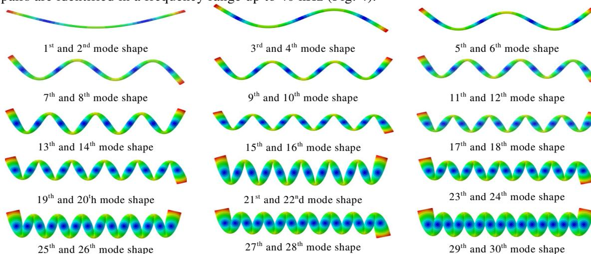
Figure 4 - First 30 bending mode shapes of an undamaged test object
