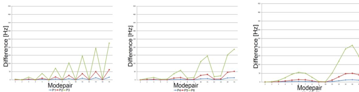
Figure 3 - Difference of numerical eigenfrequencies for the first 15 bending mode shapes (left: models 1 – 3, center: models 4 – 6, right: models 7 – 9)
