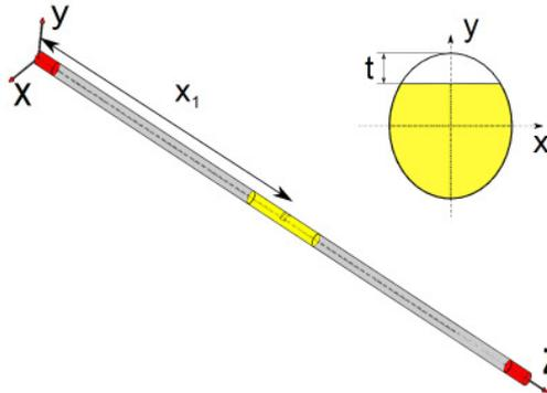
Figure 7 - Parametric model for damage identification
