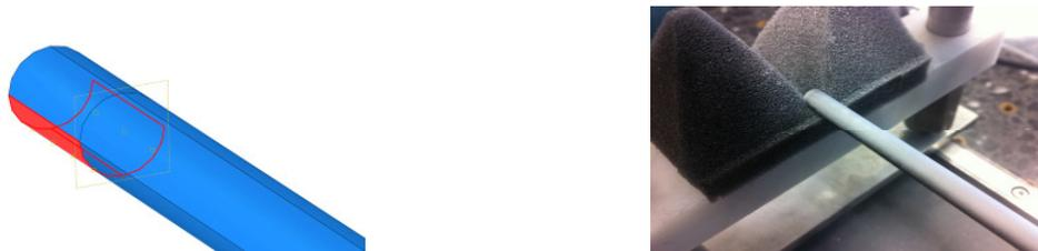
Figure 6 - Numerical and experimental support conditions
