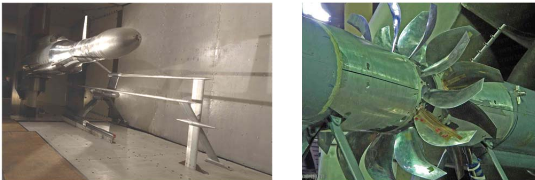
Figure 7: DREAM CROR designs in ARA (left) and TsAGI (right) wind tunnels
