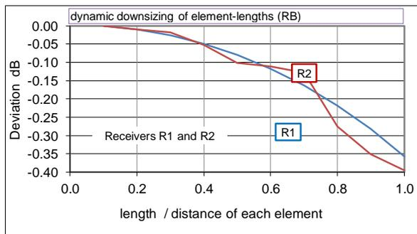
Figure 7 – Deviations caused by the size of the elements applying the RB-method
