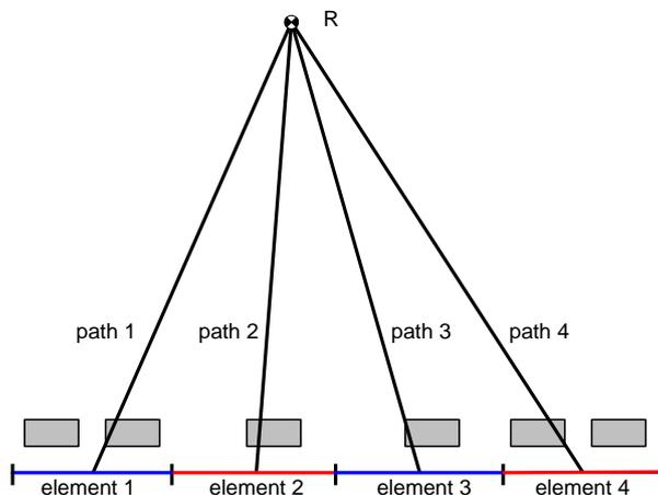
Figure 10 – A row of buildings between the line source and the receiver
