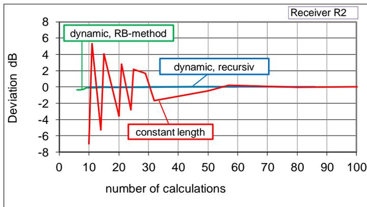
Figure 9 – Comparison of the methods by relating the deviations to the number of calculations
