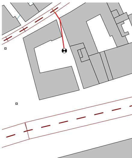
Figure 20 – Receiver with a deviation of - 12 dB if projection is not applied (only the path shown is detected without projection)
