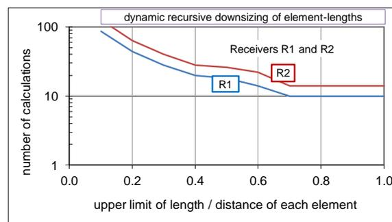
Figure 6 – Number of calculations needed with the recursion method
