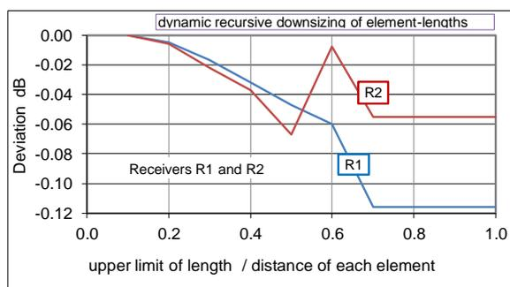
Figure 5 – Deviations caused by the size of the elements applying the recursion-method
