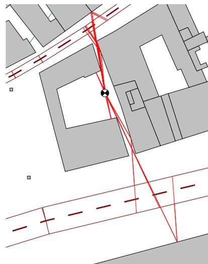
Figure 21 – same as figure 18, but paths detected with projection (the paths shown include reflection of 1st order not detected without projection)
