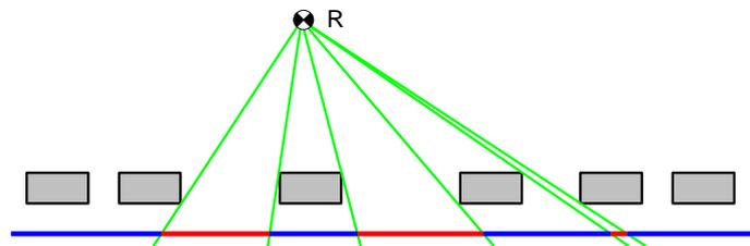
Figure 11 – Subdividing the line source by applying the projection method (first step)
