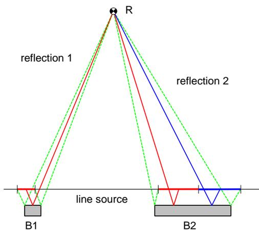
Figure 16 – The application of the projection method with reflected sound
