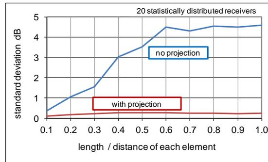
Figure 14 – The spread of deviations from the reference result over all receivers in dependence of the resolution  $k$
