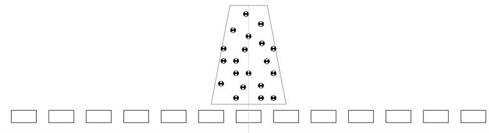
Figure 13 – Randomly distributed receivers behind a row of buildings with gaps of 10 m
