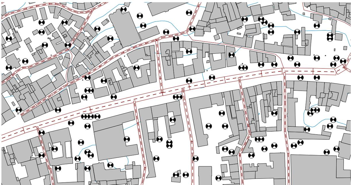
Figure 15 – 100 receivers distributed randomly in a typical inner-city-environment
