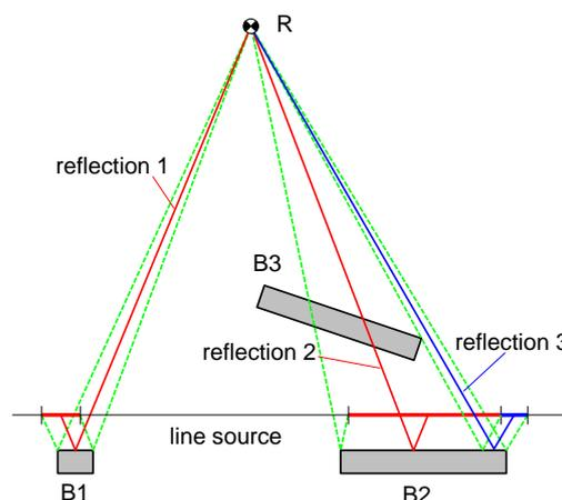
Figure 17 – Projection of reflected sound with screening object
