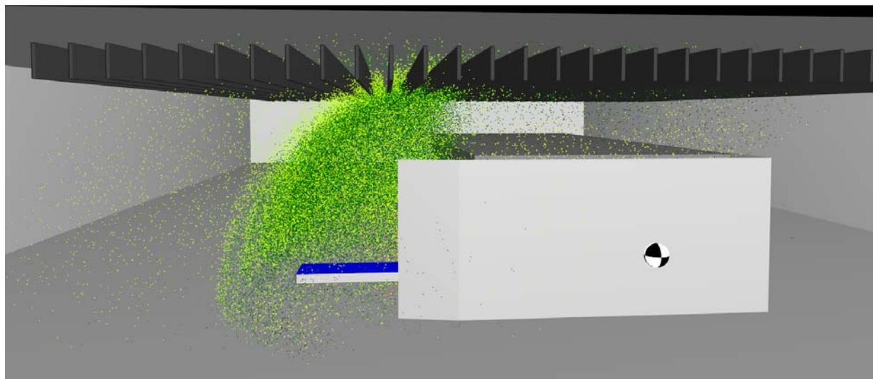
Figure 11 - Absorbing baffle structure above the machine (each baffle modeled as separate absorbing object)
