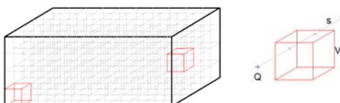
Figure 8 - Subdivision of the room in “voxels” to count the crossing particles
