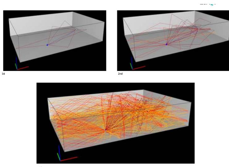
Figure 1 - Rays constructed with the mirror image method
