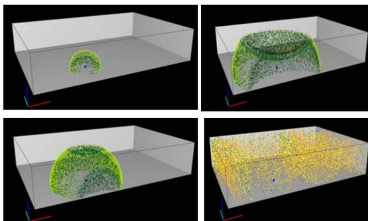
Figure 2 - Sound propagation simulated with the particle method
