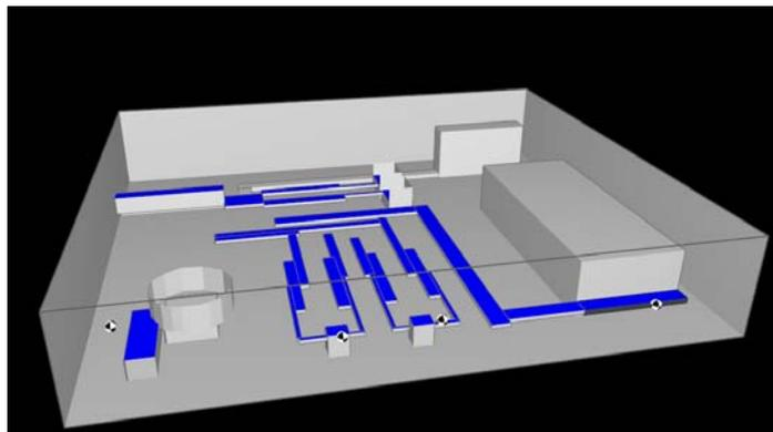
Figure 13 - Model of the bottling plant without any treatment of room surfaces
