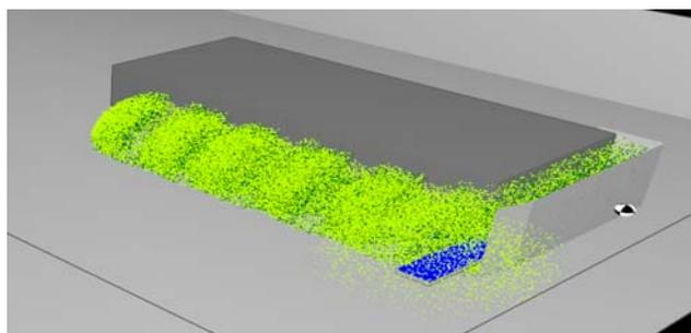
Figure 10b - Sound particles reflected by the screen
