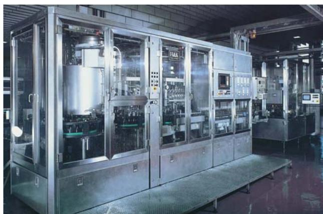
Figure 4 - Filling machine in a bottling plant
