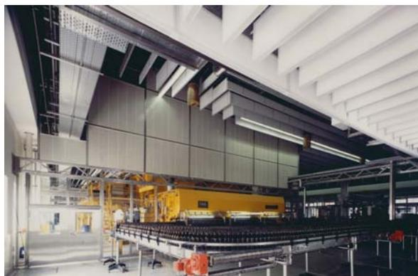
Figure 6a - Large washing machine in a bottling plant
