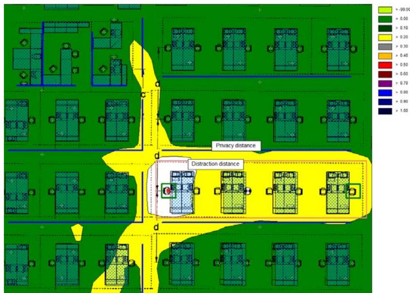
Figure 17 - Distraction distance and Privacy distance around a work place based on the calculated STI
