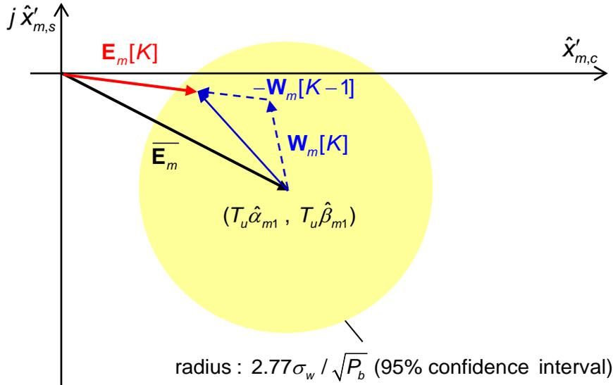
Figure 2 – The conceptual diagram of error dynamics in quasi-periodic case
