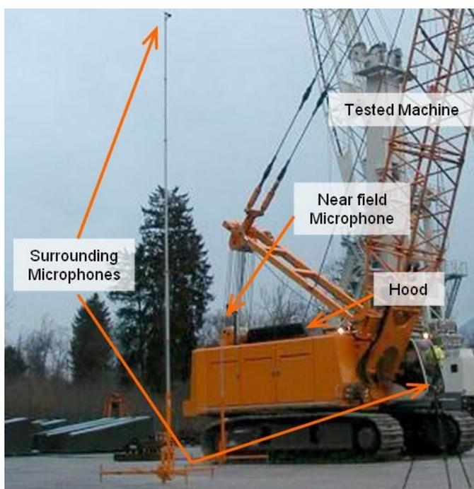
Figure 13 - Microphone positions according to European directive 2000/14/EG [4]
