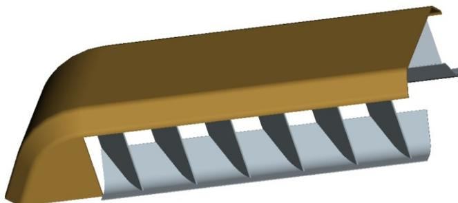
Figure 16 - Concept of a future lightweight GFRP hood
