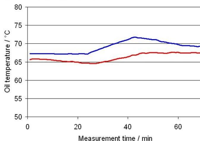
Figure 15 - Resulting oil temperature for the steel (blue) and the GFRP (red) hood during the same load case
