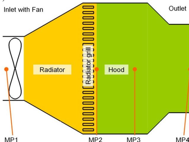
Figure 8 - Schematic draft of the measuring point for the calculation of the needed free cross section at the outlet
