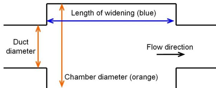
Figure 5 - Schematic draft of a reflection silencer
