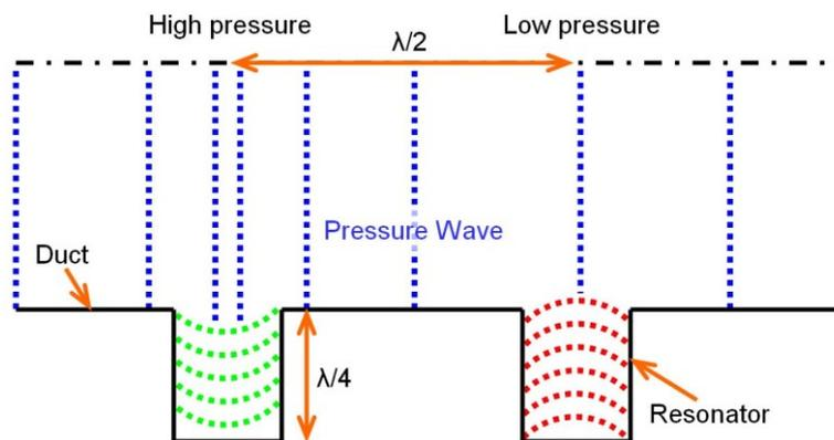
Figure 6 - Schematic draft of a  $\lambda/4$  resonance silencer
