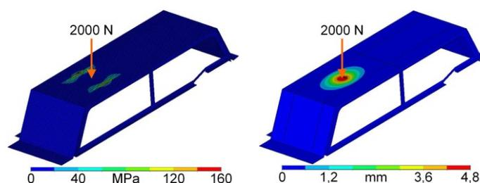
Figure 11 - Resulting equivalent stress (left) and deformation (right) for the spotty load case at the redesigned GFRP-hood
