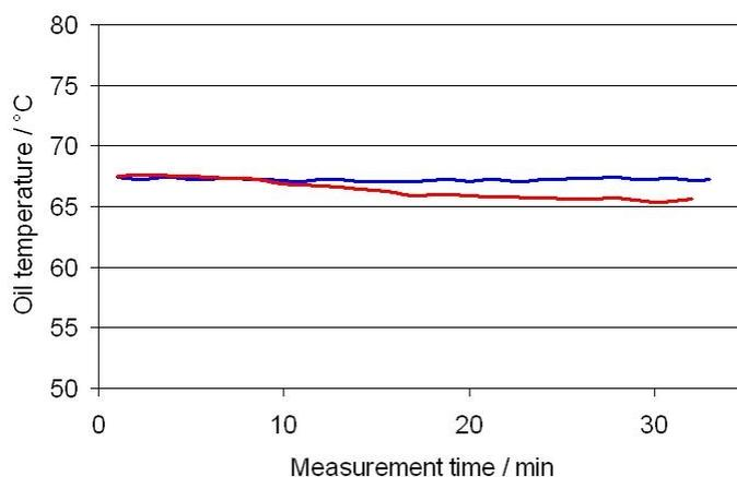
Figure 9 - Comparison of the oil temperature for different sizes of free cross section areas for the current hood (blue line - standard configuration, red line – modified configuration with reduced cross section)
