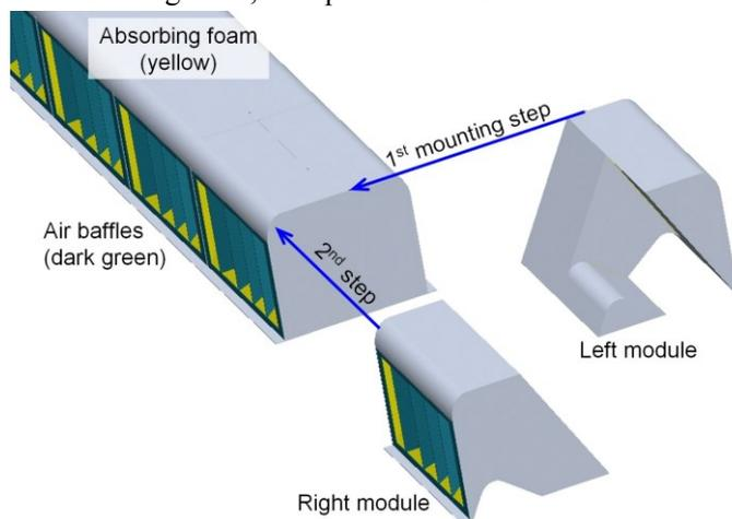
Figure 17 - Modular concept of a GFRP hood with extended flow path and additional absorbing materials inside
