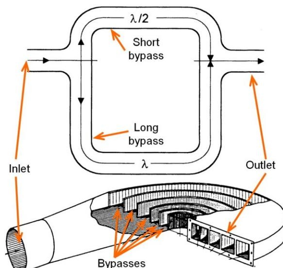
Figure 7 - Schematic draft and example of an interference silencer [3]
