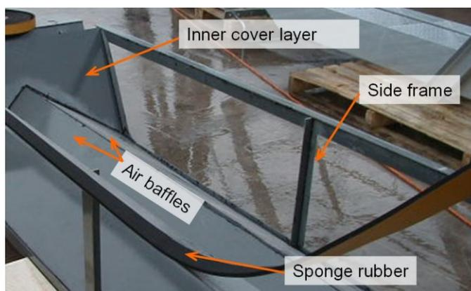
Figure 12 - Final assembly of the GFRP hood
