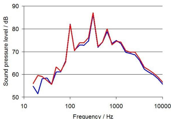
Figure 14 - Resulting sound pressure level for the steel (blue) and the GFRP (red) hood during the same load case
