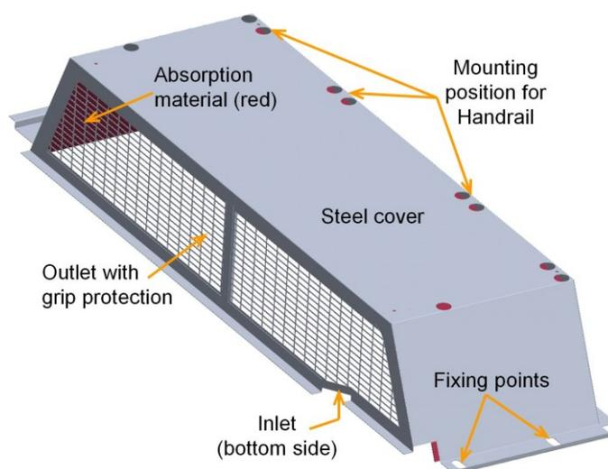
Figure 1 - Model of chosen reference hood made of steel with mounted absorption panels
