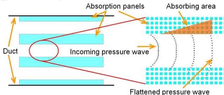
Figure 3 - Schematic draft of sound absorbing mechanism in an absorption silencer
