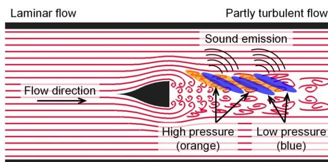
Figure 2 - Schematic draft of sound generation within a fluid flow
