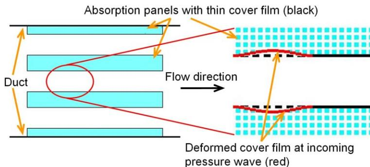
Figure 4 - Schematic draft of sound energy harvesting in a relaxation silencer
