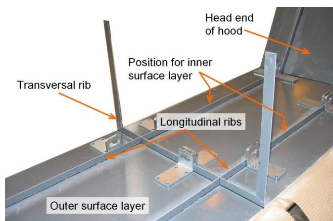
Figure 10 - Lightweight structure of the GFRP-hood
