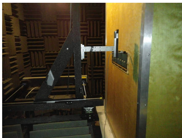
Figure 4 – Traversing single microphone setup in front of a model building located in an anechoic chamber for the accurate testing of NAH algorithms.
