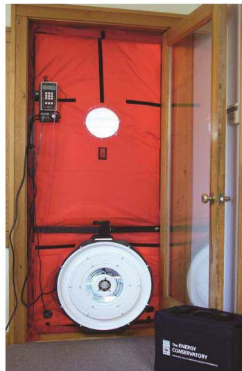
Figure 3 – A photograph of the experimental setup showing the pressure gauge and blower fan mounted on the door.
