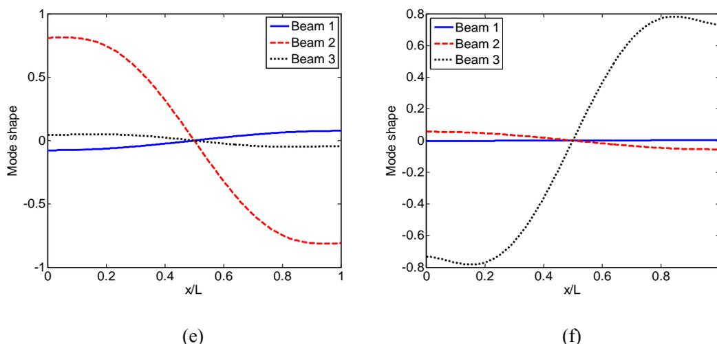
Figure 4 – The first six mode shapes for the three-beams with case 3 boundary conditions ( $K_{12}=K_{23}=1\times 10^5 N/m^2$ ,  $k_{12}=k_{23}=0$ )
