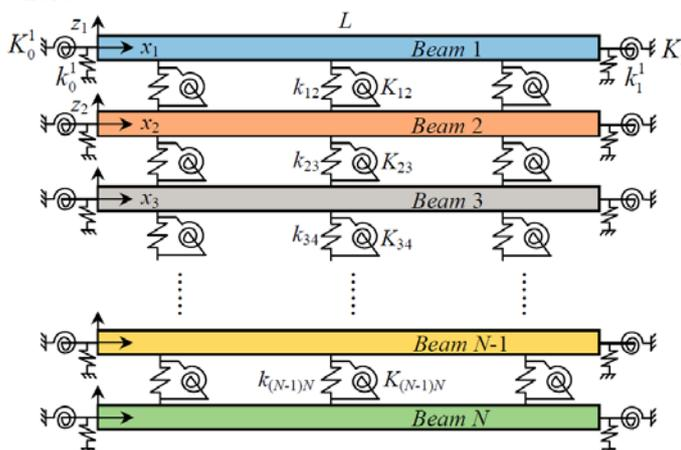
Figure 1 Elastically connected multiple-beams with arbitrary boundary conditions
