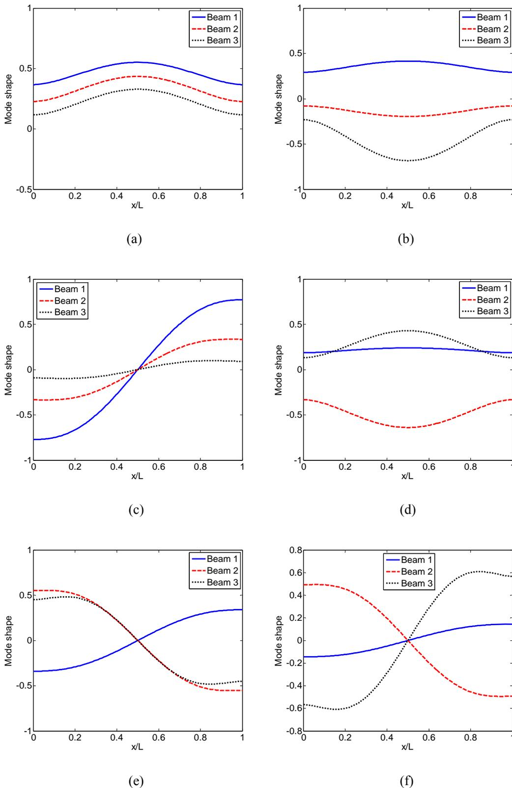
Figure 3 – The first six mode shapes for the three-beams with case 3 boundary conditions ( $k_{12}=k_{23}=1 \times 10^5 N/m^2, K_{12}=K_{23}=0$ )
