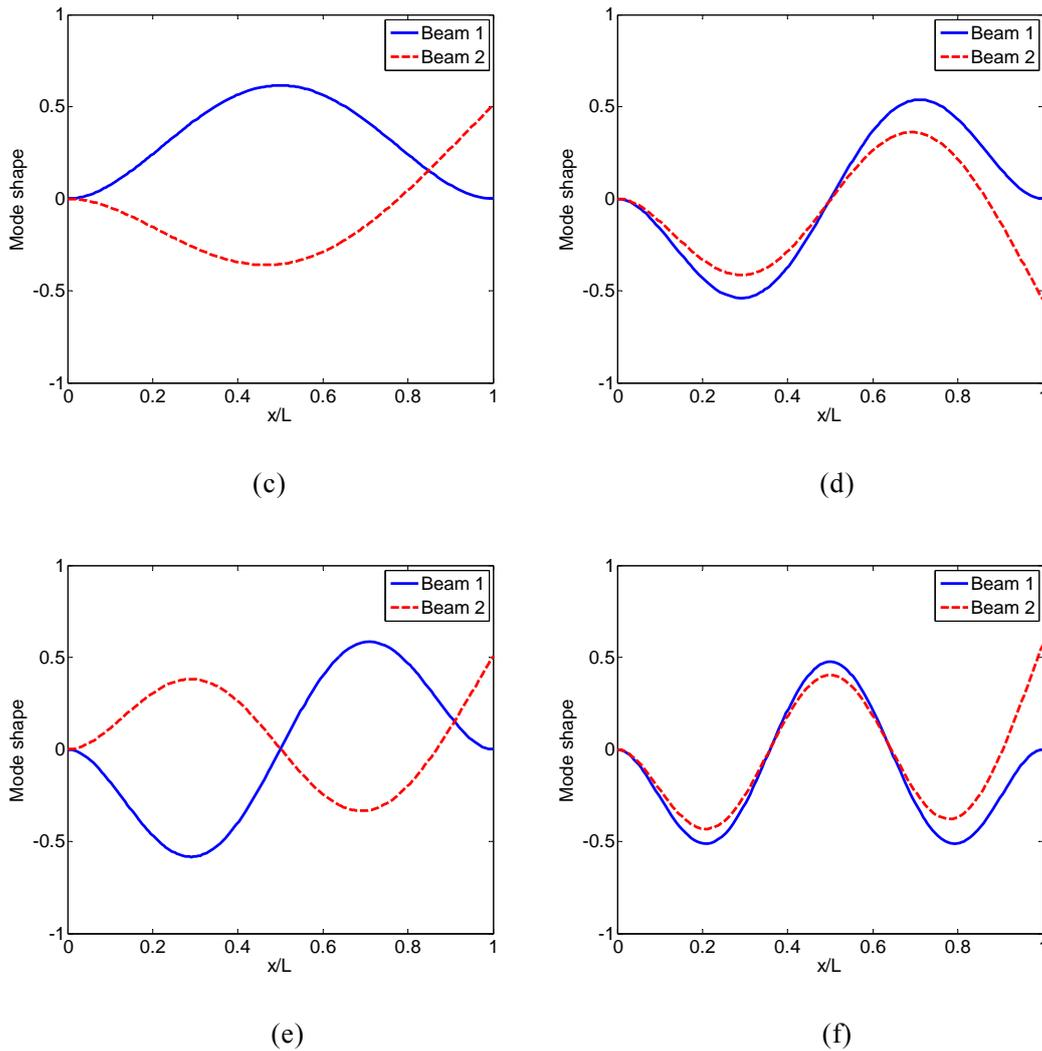
Figure. 2 Mode shapes of C-C and C-F double beam system, with rotational elastic restraint as  $K=1 \times 10^5 N/m^2$
