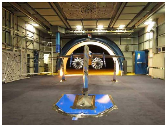
Fig. 1: Test set-up in Pininfarina WT (rear view of the aircraft model)
