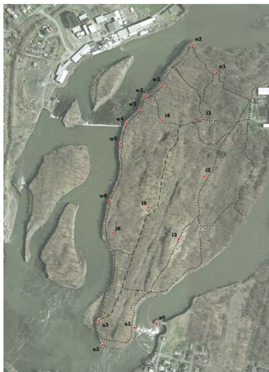
Figure 10 – This Google Earth photo of Peebles Island State Park in Cohoes, NY, is overlaid with the locations where cross-modal soundscape recordings have been made to analyze the complex combined effects of broadband waterborne sound from dams and waterfalls, and industrial machine noise from the paper plant to the north, along with surrounding forest sounds and distant roadway noise.
