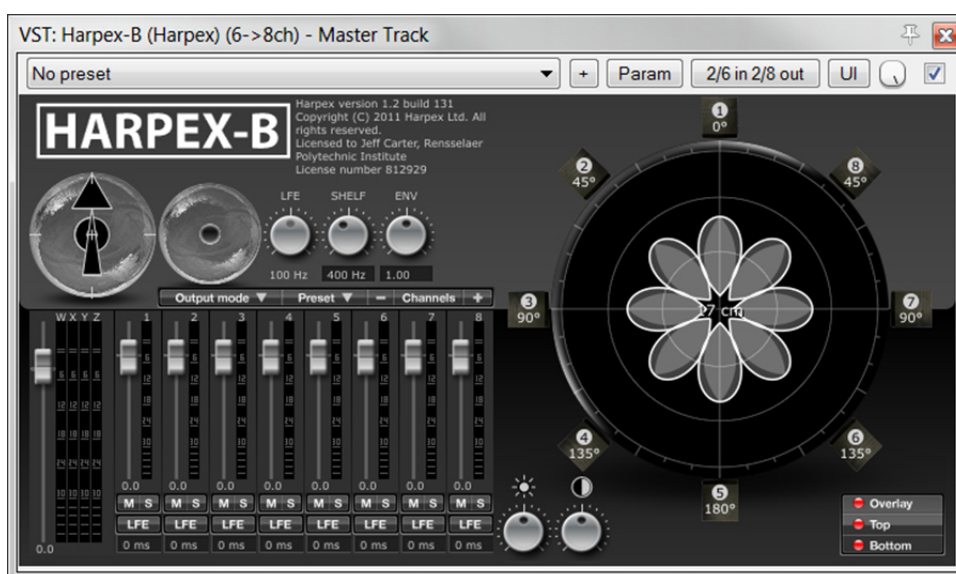
Figure 6 – Screenshot of Svein Berge’s HARPEX-B plug-in which is capable of deriving eight virtual shotgun microphones per processing pass from a single A-format capture.
