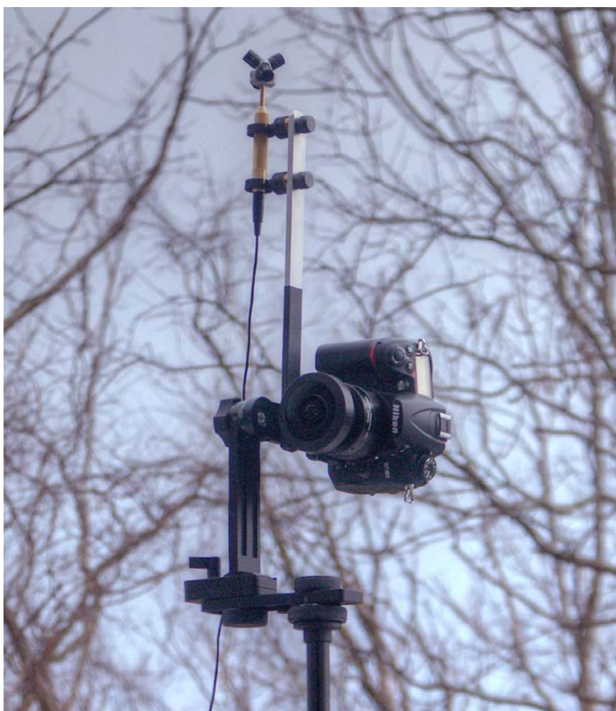
Figure 1 – Image of author’s cross-modal soundscape recording configuration comprised of Ambisonic audio capture and spherical panoramic photography.
