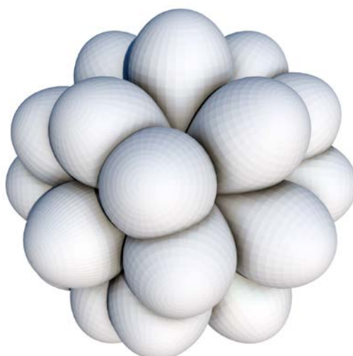
Figure 7 – With four processing passes of the A-format audio data through HARPEX-B, it is possible to approximate the above pickup pattern with 26 channels of directional shotgun feeds.
