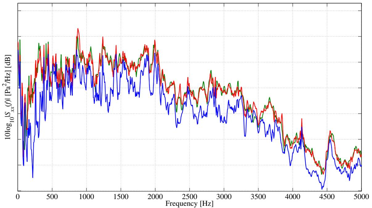
Figure 6 – Power spectral densities of the low gear rattle measurement (blue), high gear rattle measurement (green), and high gear rattle simulation (red). Each tick mark is a 5 dB increment.
