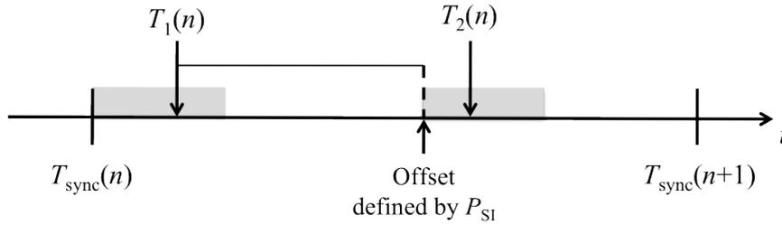
Figure 3 – Illustration of setting gear rattle impact times. The shaded areas represent the possible locations of the gear rattle impact events due to the random delay.
