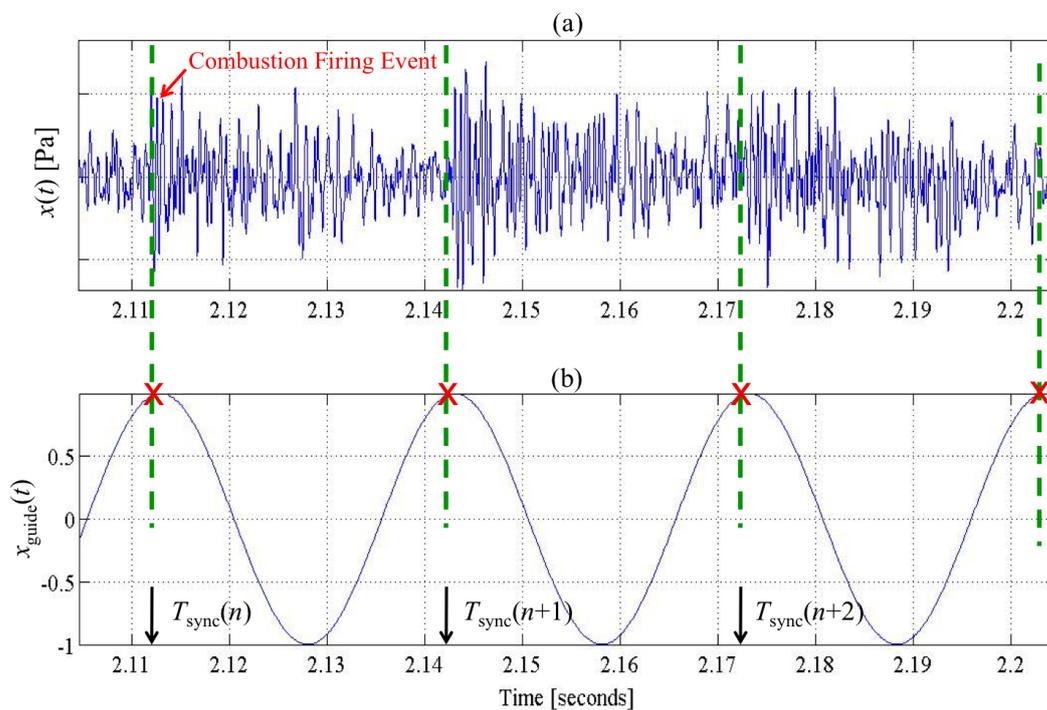
Figure 2 – Synchronizing the gear rattle primary pulse train with the (a) baseline noise measurement by using (b) a sine wave with a frequency variation of the instantaneous engine speed.
