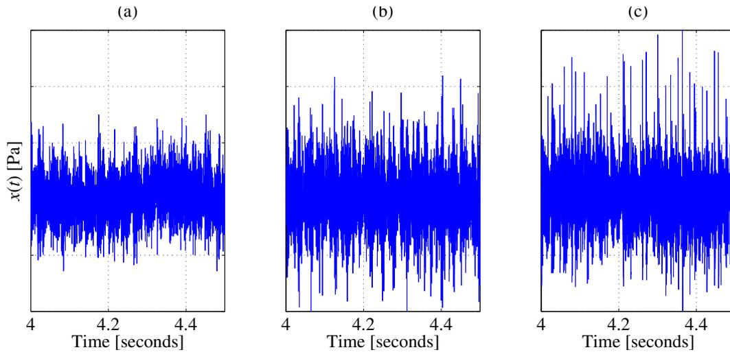
Figure 5 – The time histories of (a) the low gear rattle measurement, (b) the high gear rattle measurement, and (c) the high gear rattle simulation.
