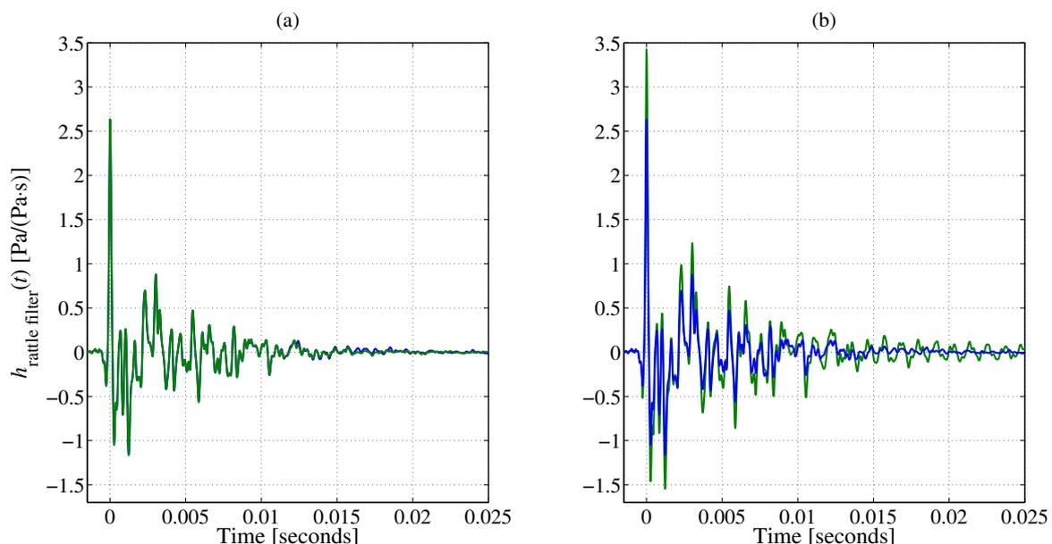
Figure 4 – (a) The original gear rattle impulse response (blue) and the Prony series model (green) and (b) the original gear rattle impulse response (blue) and the impulse response with decreased damping of various components (green). See Table 1 for parameter values.
