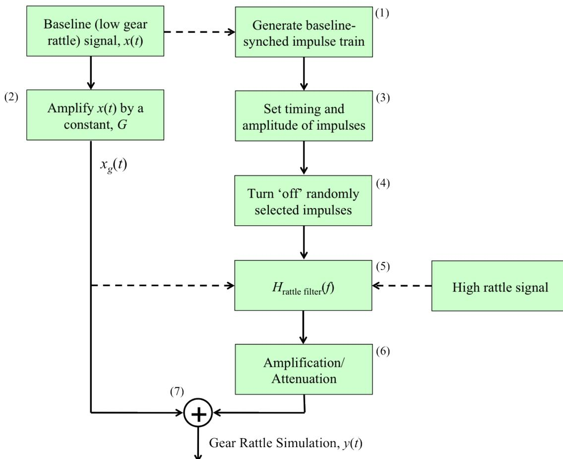
Figure 1 – Gear rattle noise simulation model.
