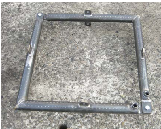
Figure 2.3.1 - One level of the multi-stage bubble ring
