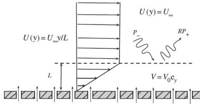
**Figure 1.** Sound propagation in a linear shear and cross layer profile.
