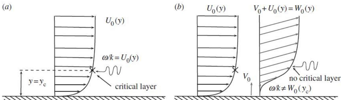
**Figure 2.** Graphical explanation of the existence of the critical layer. (a) Acoustic propagation in pure shear flow. (b) Acoustic propagation in shear and cross-flow.
