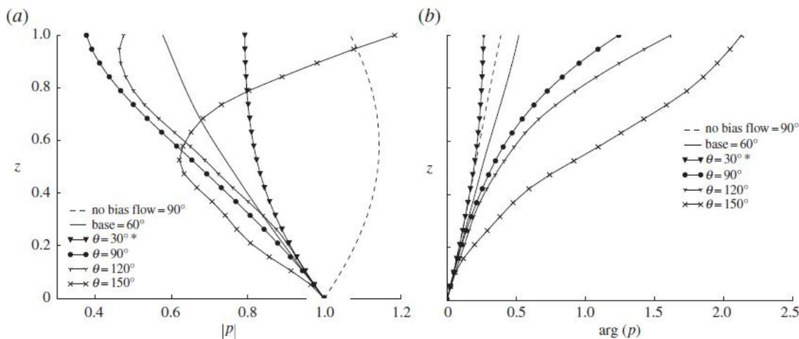
**Figure 3.** For five values of the angle of incidence is plotted the (a) modulus and (b) phase of acoustic pressure versus dimensionless distance from the wall (4.4a) the pressure is also normalized to the wall value. The free stream Mach number (4.8b) is  $M_\infty = 1.2$ , the bias flow Mach number (4.8a) is  $M_0 = 0.05$  and the dimensionless frequency (4.8a) is  $\Omega = 1$ . The wall specific impedance is  $Z = 1 + i$ .
