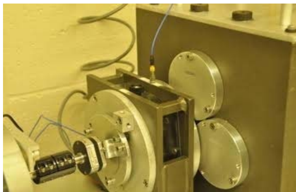
Figure 3. Accelerometer mounted on the gearbox to measure vibration signals.
