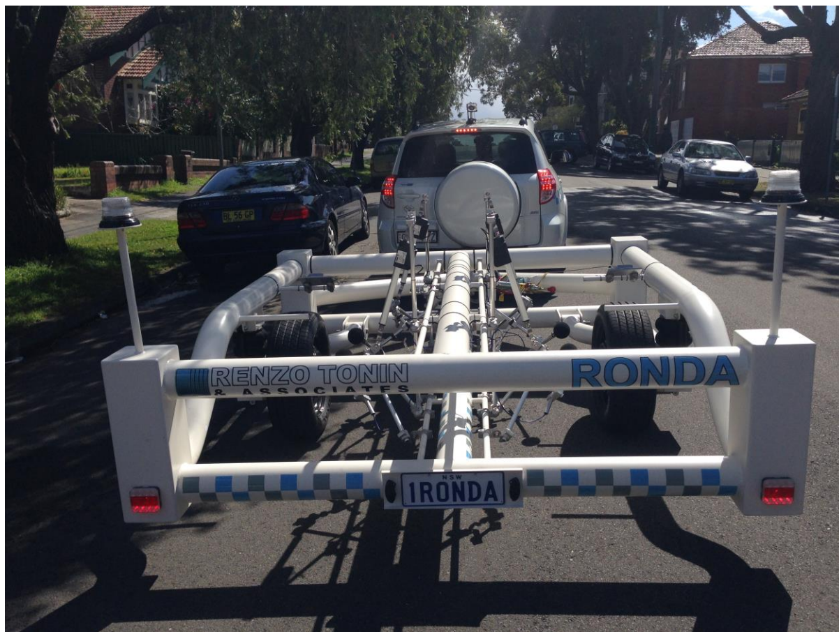
Figure 3 View of RONDA showing microphone frame support structure
