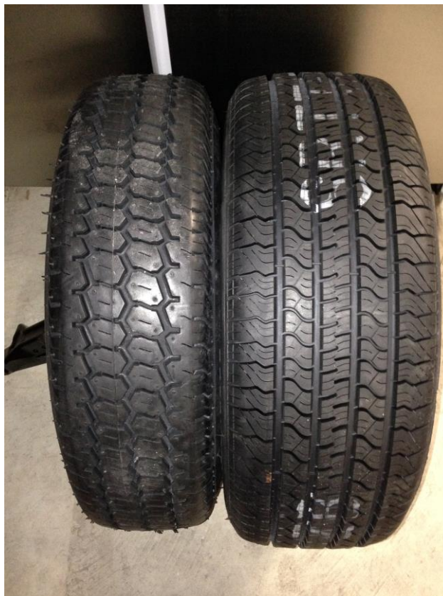
Figure 1 Standard Reference Tyres: 14" Avon 4 (left) and 16" SRTT (right)
