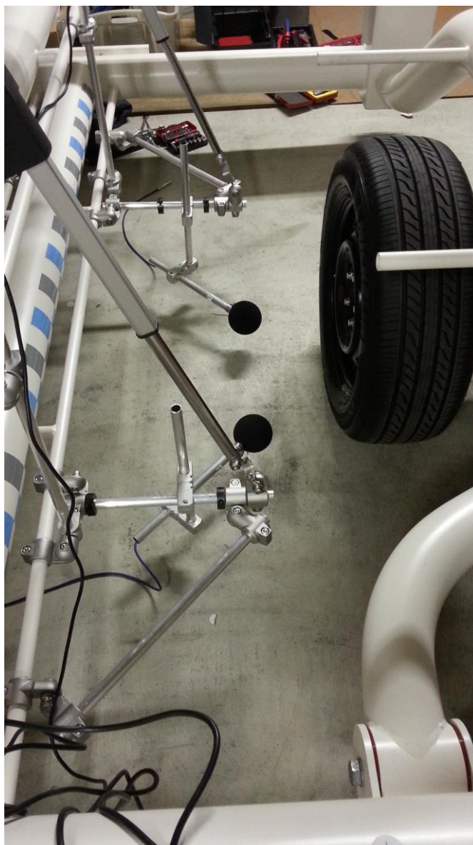
Figure 4 Microphone frame support structure for the left hand tyre viewed from front of trailer
