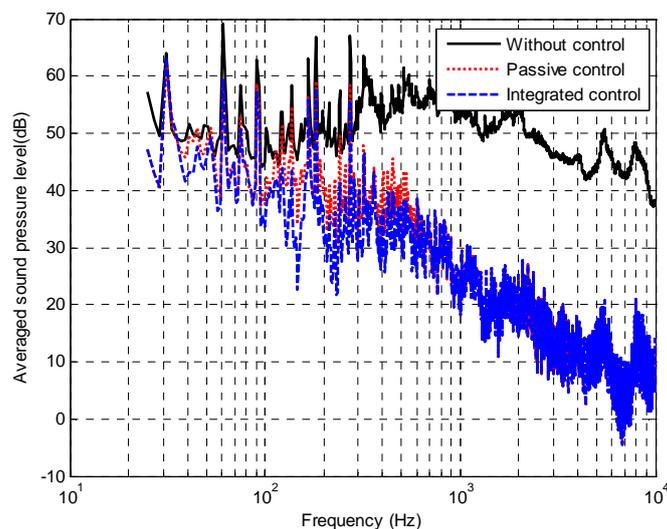
Figure 10 - Spatially averaged noise spectra of various control modules for engine noise without weighted
