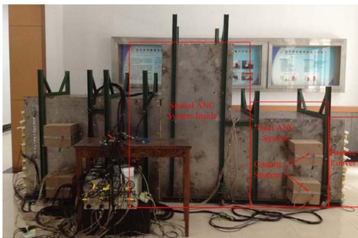
Figure 2 – A photo of the integrated passive and active control system.
