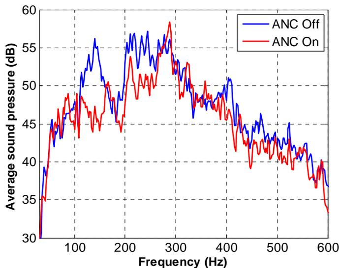
Figure 9 - Spatially averaged engine noise spectra with and without the integrated active noise control
