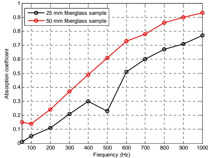
Figure 4 – Sound absorption coefficients of two fiberglass samples.
