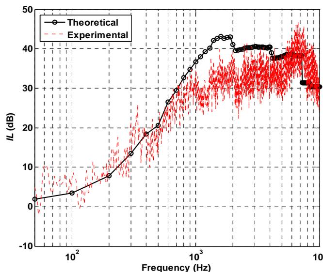
Figure 3 - Measured and predicted insertion losses of the passive enclosure.
