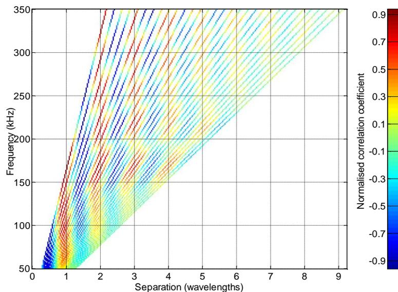
Figure 3 – The correlation of thermal noise travelling through water between two hydrophones.
