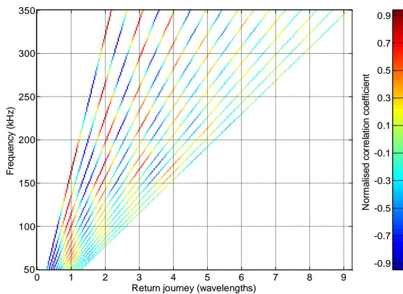
Figure 2 – The auto-correlation of thermal noise travelling through water between a hydrophone and wall boundary.
