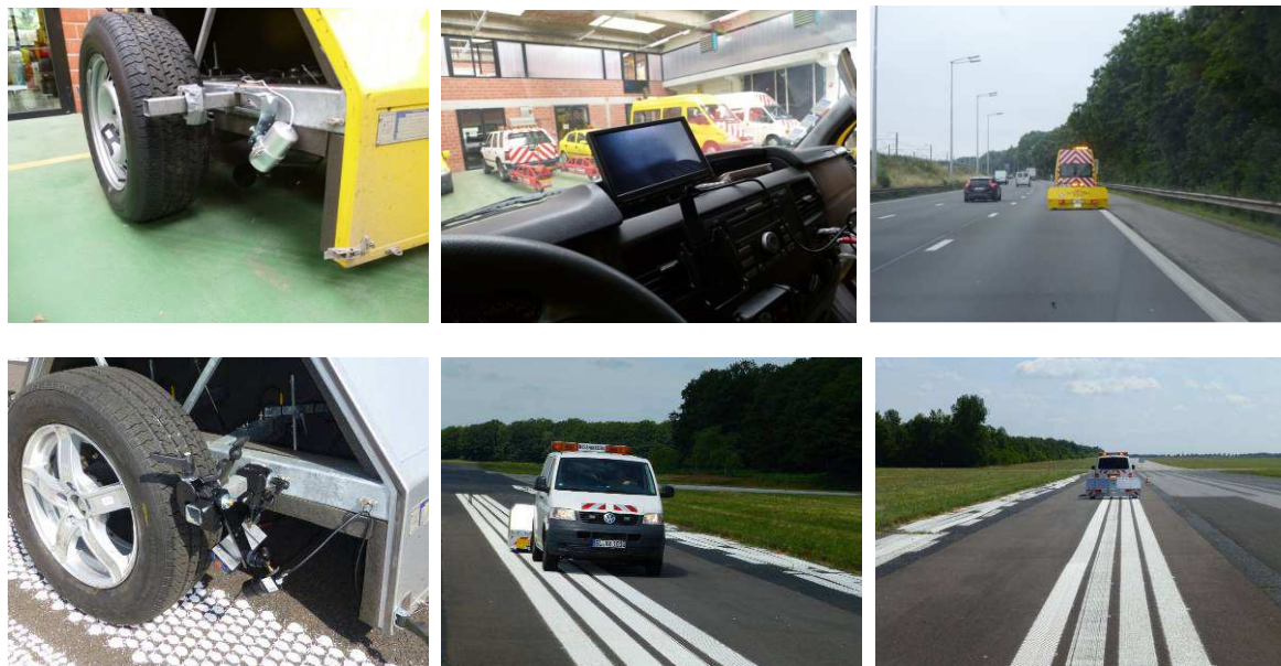
Figure 3 – The CPX trailers with modifications for measuring on audio-tactile road markings (left and middle) and such measurements (right hand side). Upper row: CPX trailer of the Flemish Agency for Roads and Traffic. Lower row: CPX trailer of the German Federal Highway Research Institute.
