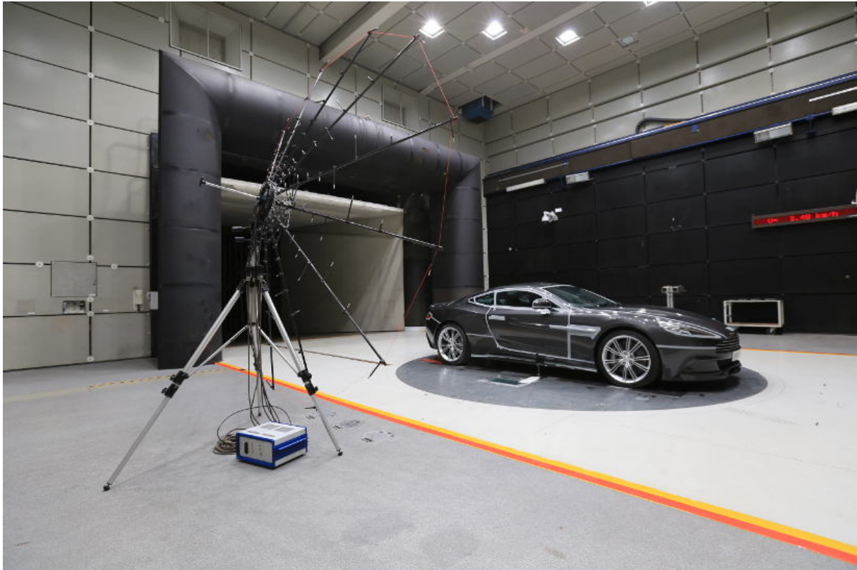
Figure 1 – Spiral array, positioned outside the shear layer.
