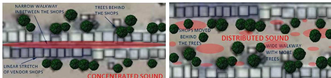
Figure 14- Existing arrangement of Vendor shops (left), Suggested arrangement to reduce noise (right)
