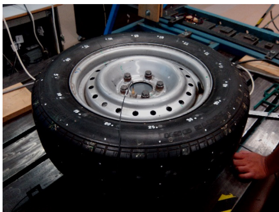
Figure 2 – Tyre-rim assembly setup for roving impact tests
