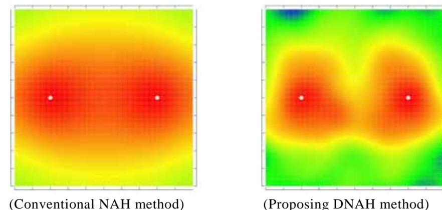
Figure 8 – The numerical simulation results of dual same phase point sources located at (0.2,0.5) and (0.8,0.5) .
