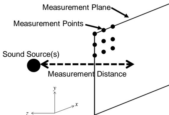
Figure 1 – This is an explanation of measurement of NAH method.
