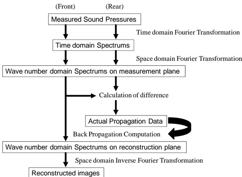
Figure 4 – This is the explanation of computation steps of reconstruction in DNAH method.
