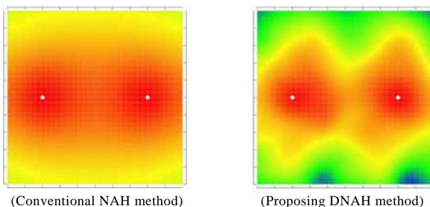
Figure 10 – The numerical simulation results of dual same phase point sources located at  $(0.2, 0.5)$  and  $(0.8, 0.5)$  .
