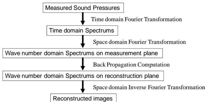
Figure 3 – This is the explanation of computation steps of reconstruction in NAH method.
