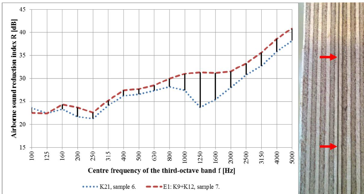
Figure 3 – Comparison of sound reduction index values of 21 mm thick plywood specimens in frequency domain on the left. Side of the glued sample, with red arrows pointing the glue line, is presented on the right.
