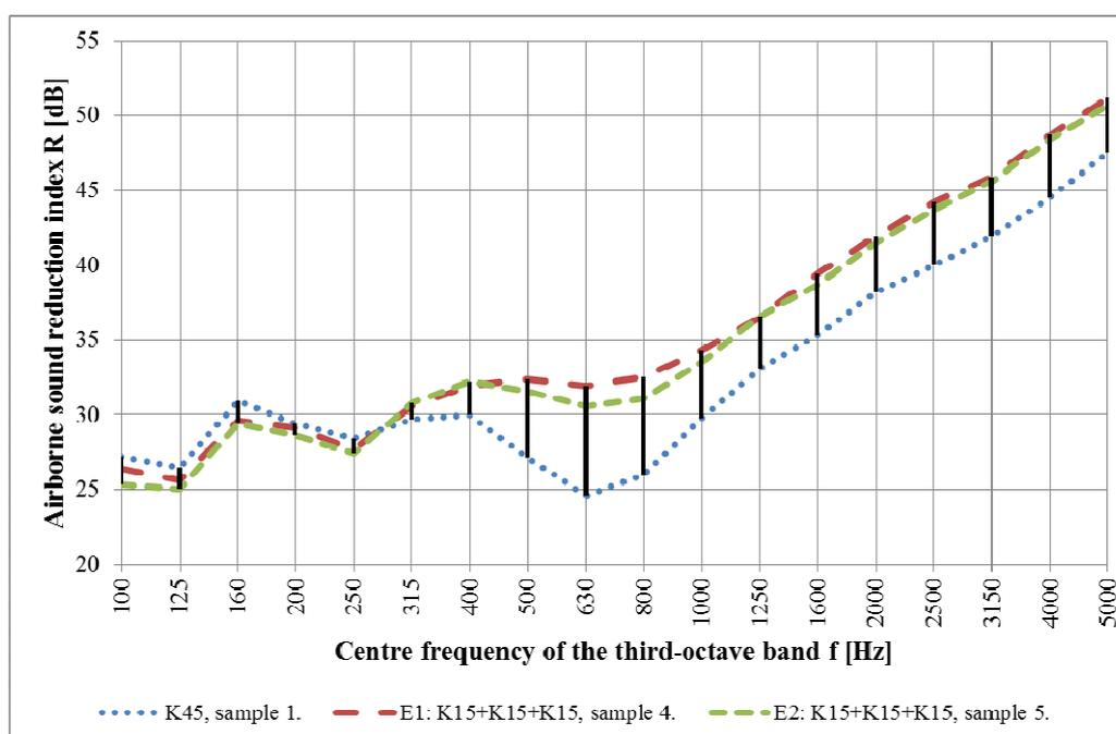
Figure 5 – Comparison of sound reduction index values of 45 mm thick plywood specimens in frequency domain. The damping glue used in samples 4. and 5. is slightly different.
