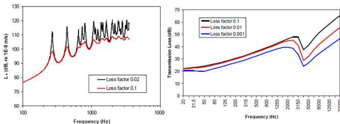
Figure 1 – The effect of damping on the mean velocity level of a structure (left) and on the transmission loss of a wall structure. [1]
