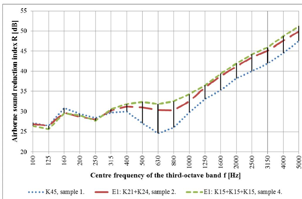
Figure 4 – Comparison of sound reduction index values of 45 mm thick plywood specimens in frequency domain.
