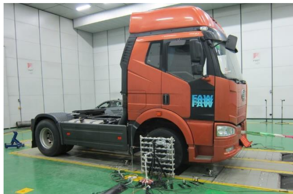
Fig. 1 Overall indoor TBR noise test setup
