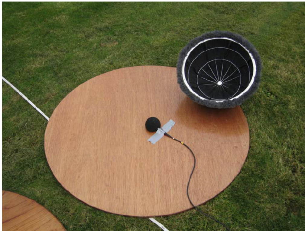
Figure 1: DELTA H Secondary Windscreen using a Wire Frame and Reinhardt Cloth [4]
