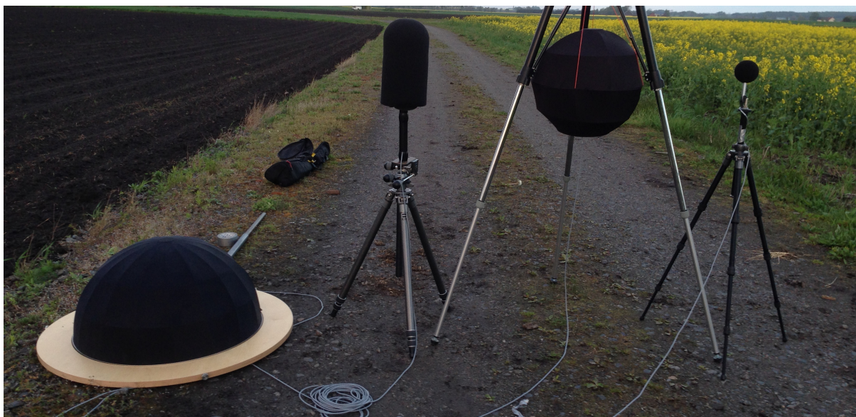
Figure 6: Photo of three Secondary (with Primary) Windscreens tested and Standard Primary Windscreen
