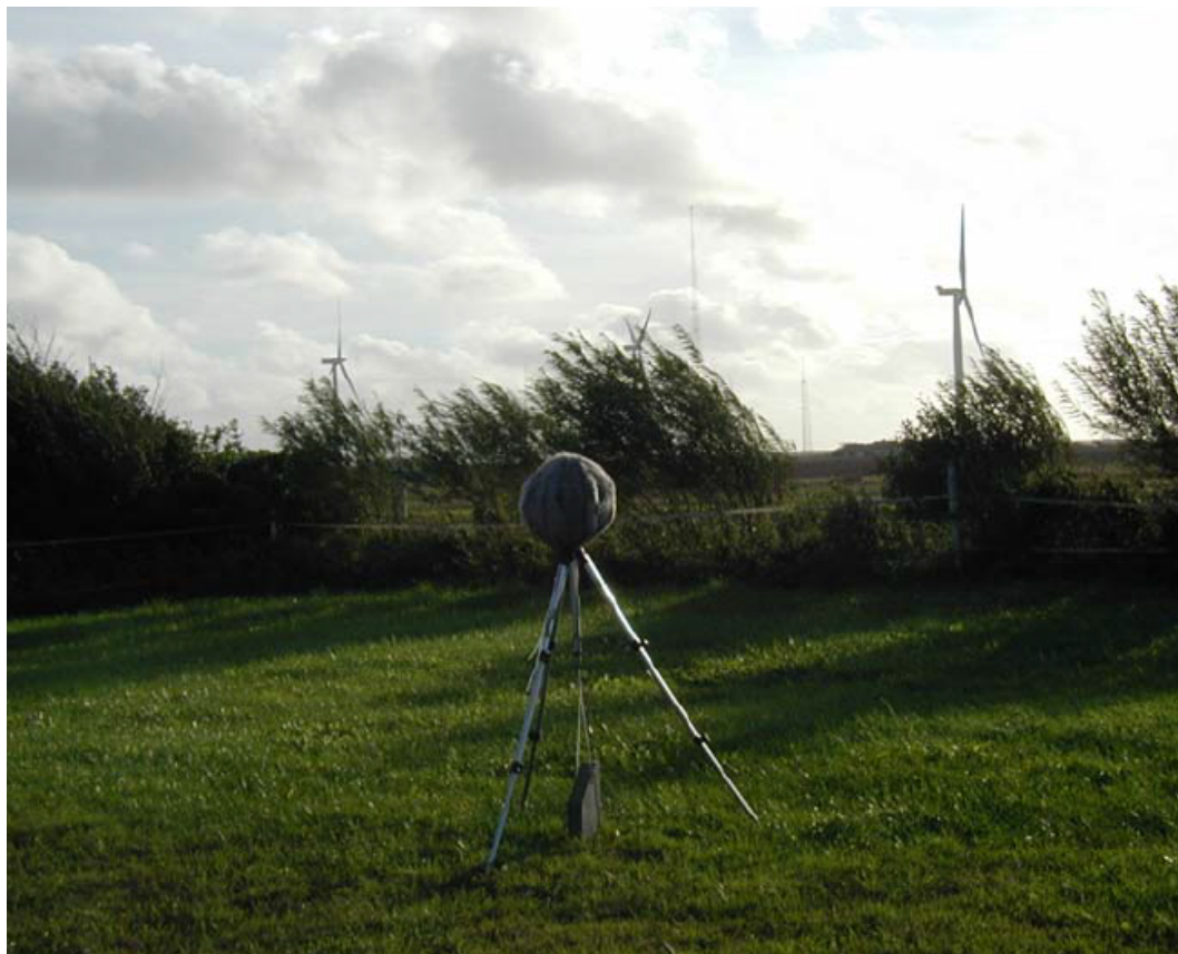
Figure 2: Immersion Measurements using a Spherical Windscreen [4]
