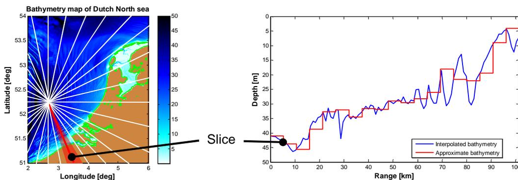
Figure 2 – Bathymetry map of the Dutch North sea divided into slices (left) and the interpolated and approximated bathymetry for a 2D bathymetry slice (right).
