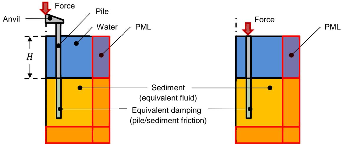
Figure 4 – Schematic overview of an FE model for a generic pile driving case (left) and the COMPILE benchmark case (right) as defined in section 3.2.
