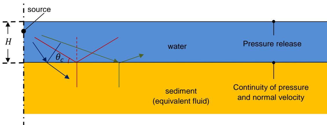
Figure 3 – Schematic geometry of a Pekeris waveguide with a point source. The green arrow represents a wave incident at angle  $\theta$  below the critical angle  $\theta_c$  (indicated by the red lines) that is fully reflected back into the waveguide (associated with propagating modes). The blue arrow represents a wave incident above the critical angle that partially transmits its energy to the sediment (associated with leaky modes).
