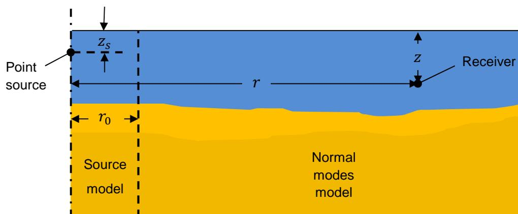
Figure 1 – Schematic geometry of a range dependent water waveguide including a (point) source and (point) receiver. The waveguide is modelled by a source and normal mode model that are coupled at  $r_0$ .
