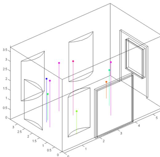
Figure 2 – Loudspeaker positions used in the qualification procedure
