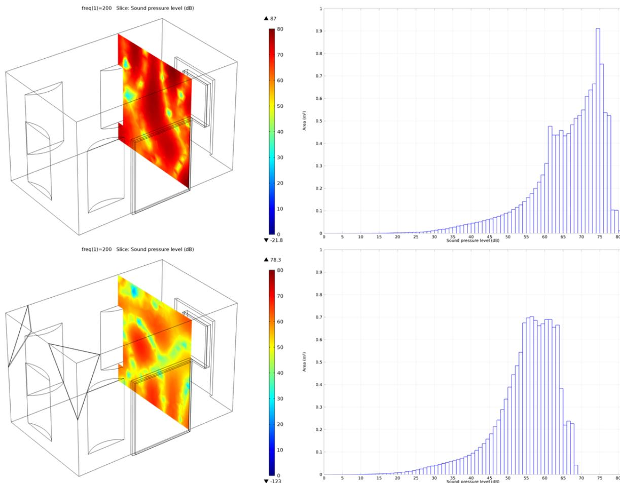
Figure 6 – Distribution of the sound pressure level at 200 Hz at the slice in the original room (upper diagrams) and with additional reflectors (lower diagrams)
