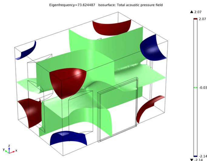
Figure 4 – Eigenmode of the room at 73.6 Hz;
