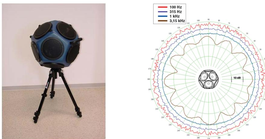
Figure 1 – Dodecahedron loudspeaker Norsonic type 270H and its directivity pattern (3). The graph shows the respons for a sinusoidal signal at 100 Hz, 315 Hz 1 kHz and 3.15 Hz in the horizontal plane through the center of the loudspeaker.
