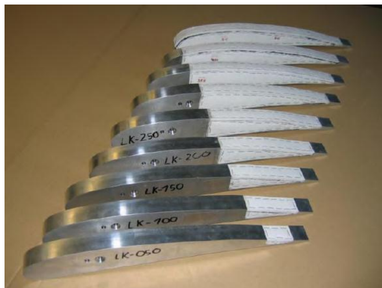
Figure 2 – Porous flap side edge treatments for assessment in wind tunnel test [7]
