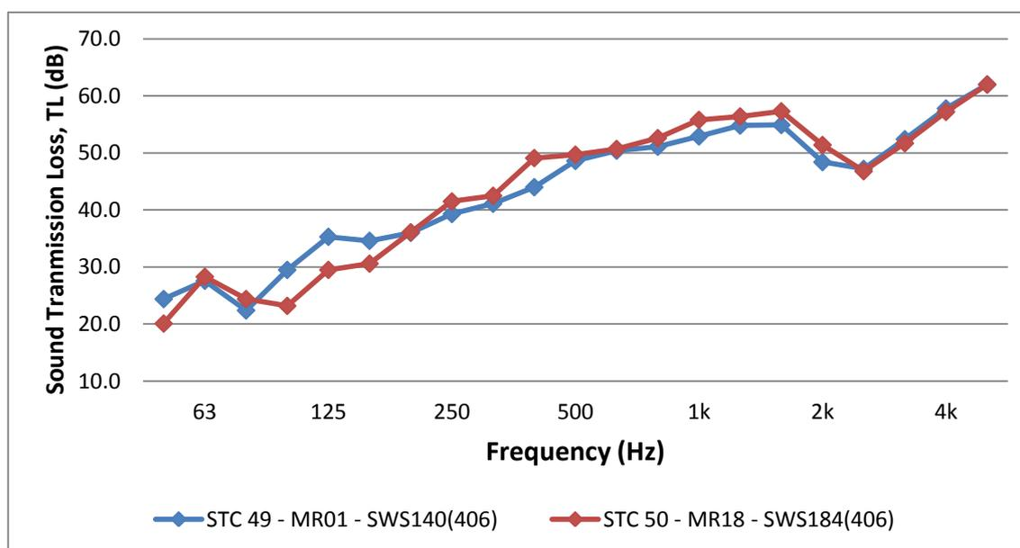
Figure 1 – Effect of stud depth on sound transmission loss. Nominally the same walls except with different stud and cavity depths (140mm and 184mm).
