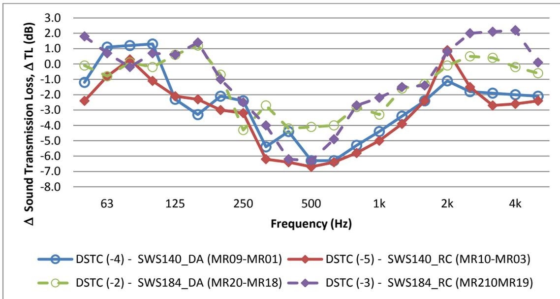
Figure 4 - Effect of end columns on sound transmission loss for different design variants: 140mm and 184mm deep cavity, and direct (DA) and resiliently (RC) mounted gypsum board.
