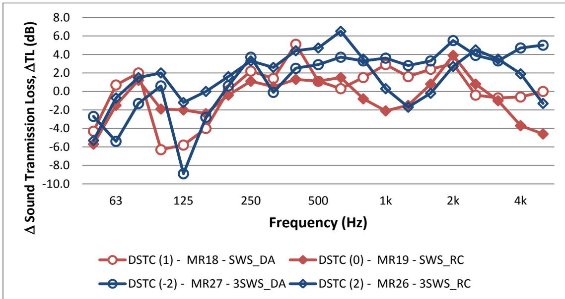
Figure 2 - Effect of stud depth on sound transmission loss for different design variants: single and tripled studs, and directly and resiliently mounted gypsum board.
