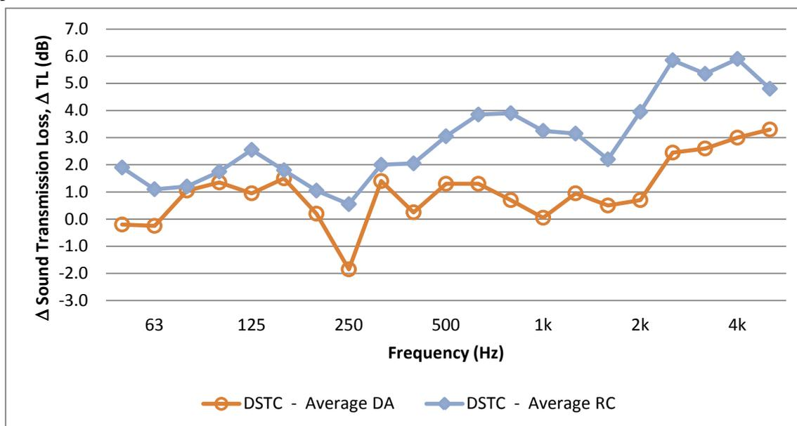
Figure 6 – Average effect of PLY16V shear membrane on sound transmission loss for direct and resiliently mounted gypsum board.
