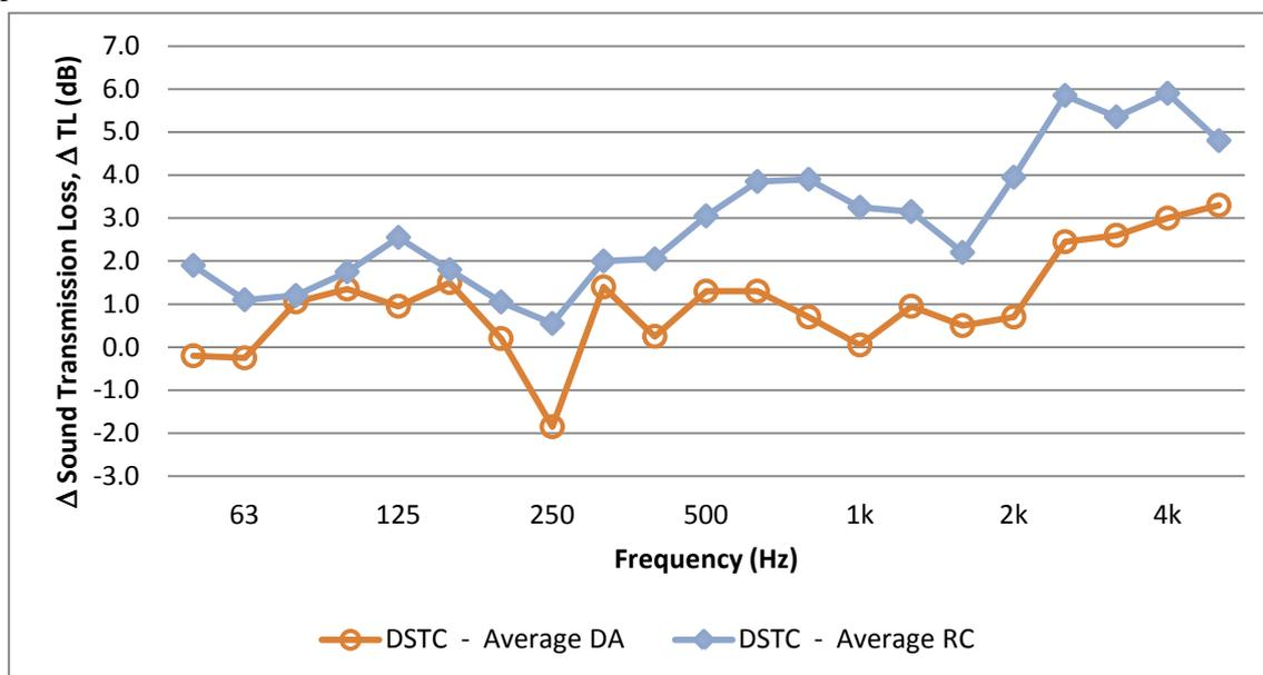
Figure 6 – Average effect of PLY16V shear membrane on sound transmission loss for direct and resiliently mounted gypsum board.
