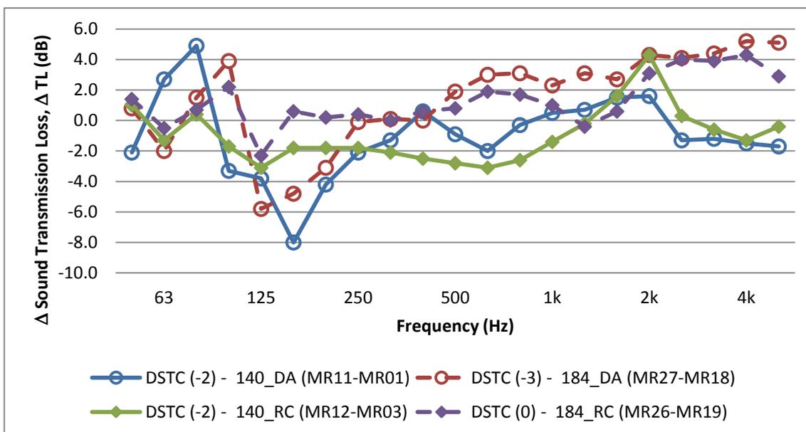
Figure 3 - Effect of stud width (single or tripled) on sound transmission loss for different design variants: 140mm and 184mm deep cavity, and direct and resiliently mounted gypsum board.
