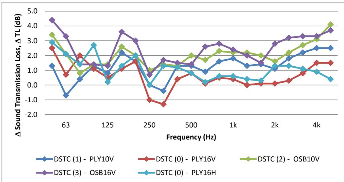
Figure 5 - Effect of shear layers on sound transmission loss for on wall MR01 with 140mm cavity depth and directly attached gypsum board.
