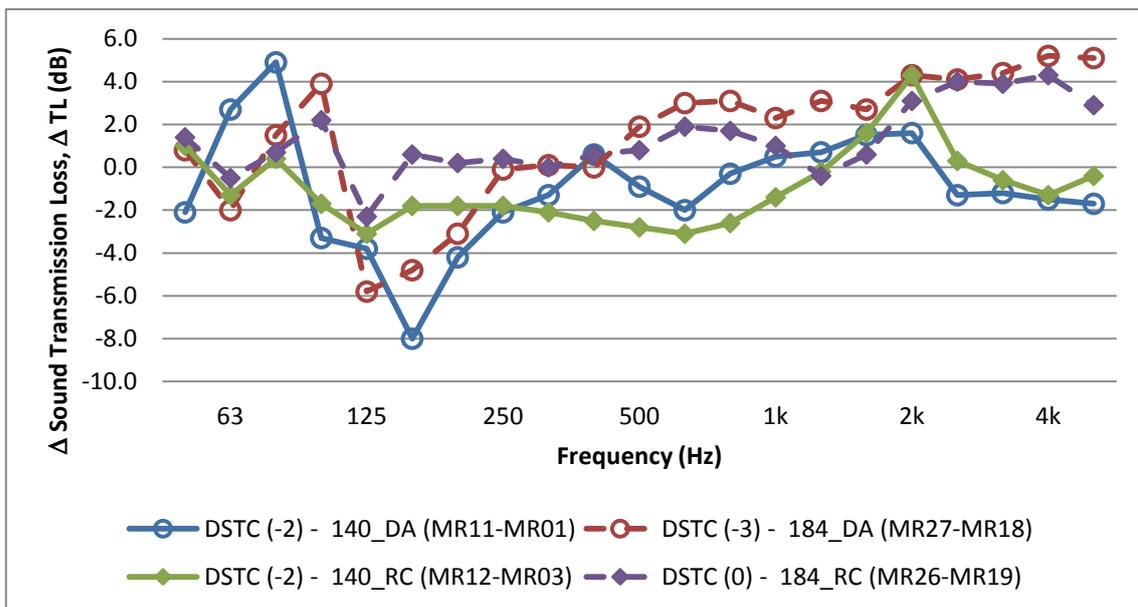
Figure 3 - Effect of stud width (single or tripled) on sound transmission loss for different design variants: 140mm and 184mm deep cavity, and direct and resiliently mounted gypsum board.
