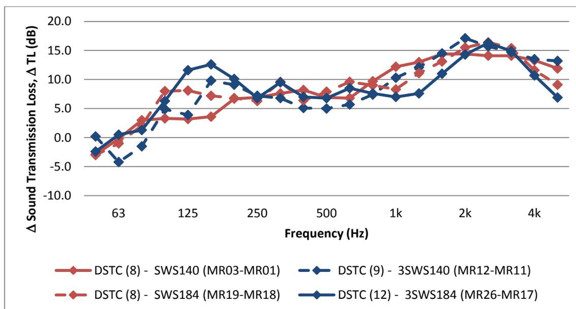
Figure 7 - Effect of resilient channels on sound transmission loss for different design variants: 140 mm and 184 mm deep studs, and single and tripled studs.
