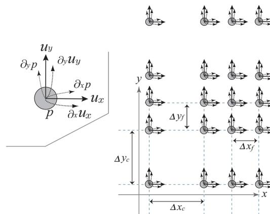
Figure 4 – Discretized acoustic field components in Non-uniform grid model
