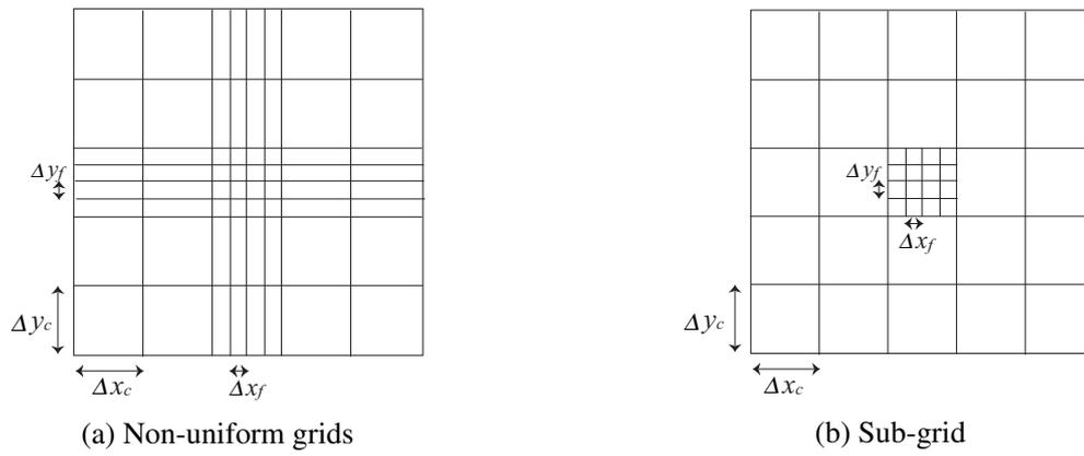
Figure 3 – Non-uniformity grid and sub-grid model
