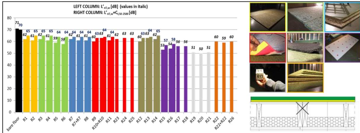
Figure 2 – Results for different type of resilient layers combined loaded with a double layer particle boards (12 mm + 18 mm as simulated parquet). The grey results approach the target limit, but are far too resilient with respect to vibrational comfort (“trampoline effect”).
