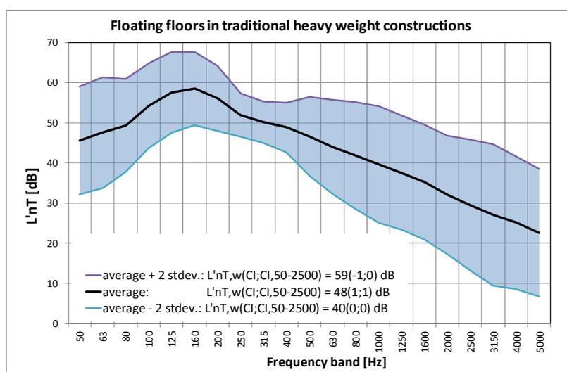
Figure 1 – Average spectrum of the standardised impact sound pressure level  $L'_{nT}$  measured in-situ on 20 well-executed traditional floating floors in Belgium. 95% of the measured values are situated inside the shaded zone
