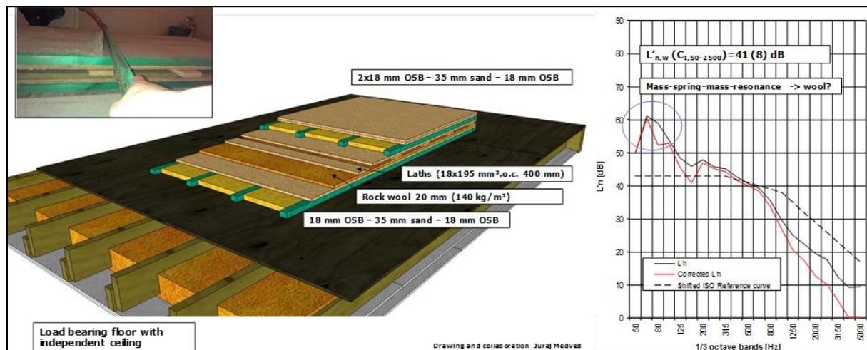
Figure 3 – Measured impact sound pressure level of two sand-filled elements put on top of a load bearing floor with independent ceiling. The upper element rests on OSB laths, put on a 20 mm rock wool mat applied on top of the lower sand-filled element. Also shown is the  $L'_n$  spectrum corrected for airborne tapping noise transmission according to ISO 10140-3:2010/FDAmd 3:2014..
