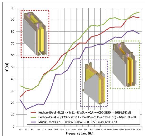
Figure 5. In-situ airborne sound insulation of double-stud party walls with panels inside the central cavity (Mobic mock-up) and with panels moved outside the central cavity (Hechtel-Eksel liv23 -> liv21). The green curve (Hechtel-Eksel slpk23 -> slpk21) shows the performance of the previous construction where at both sides a technical lining using timber battens has been added.
