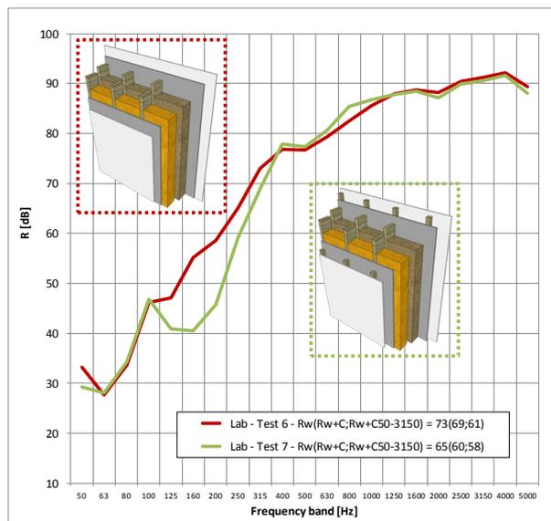
Figure 6. Laboratory airborne sound insulation of double-stud party walls with and without technical linings.
