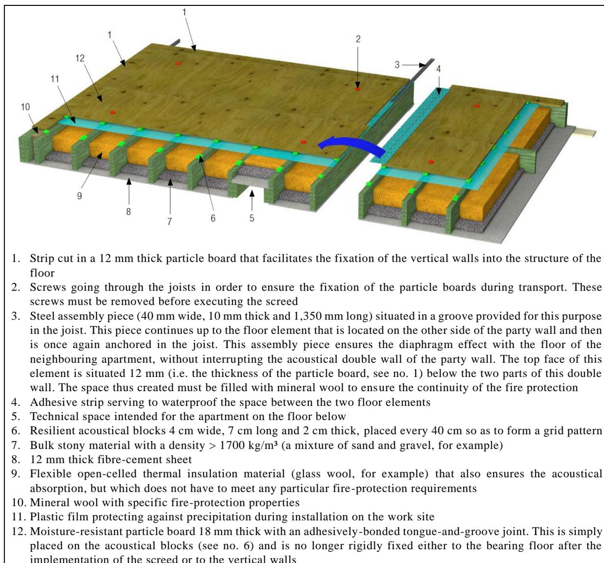
Figure 4 – Schematic drawing of the innovative LWTF floor.
