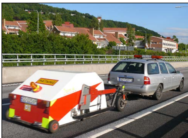
Figure 4 – CPX noise tests with the TUG Tiresonic Mk4 trailer on the DPAC pavement on E4 in Huskvarna. The test tyre is mounted in the middle of the chamber.
