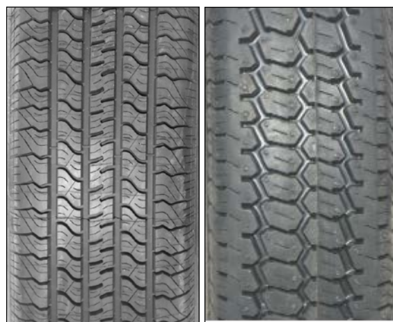
Figure 5 – Tread patterns of the two test tyres used during the CPX noise tests. From left to right: SRTT (P1) and Avon AV4 (H1).
