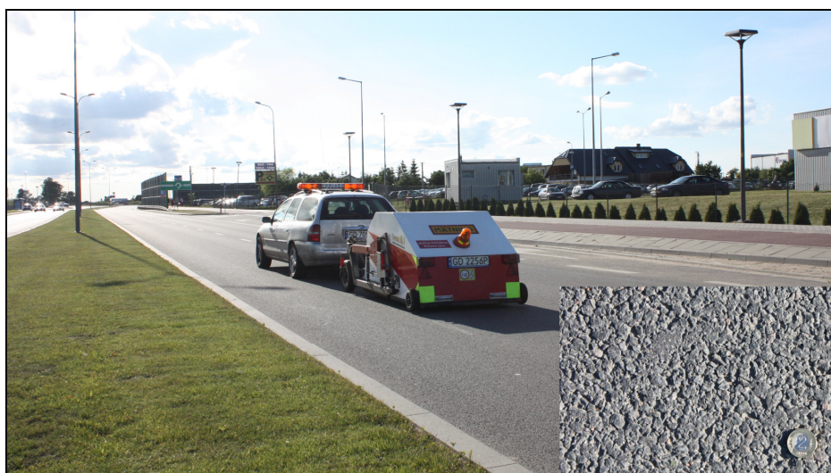
Figure 1 – The CPX test vehicle Tiresonic Mk4 at the test section and close-up of test surface (the diameter of coin is 21.5 mm)
