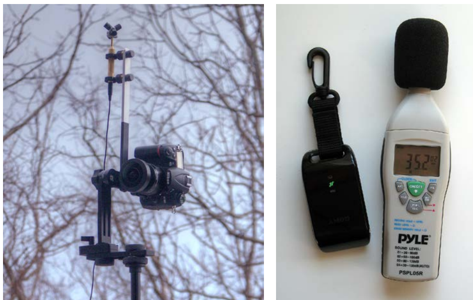
Figure 1 – Left: author's custom cross-modal soundscape recording configuration comprised of Ambisonic audio capture and spherical panoramic photography. Right: AMOD AGL3080 GPS datalogger and Pyle Pro PSPL05R digital SPL meter.
