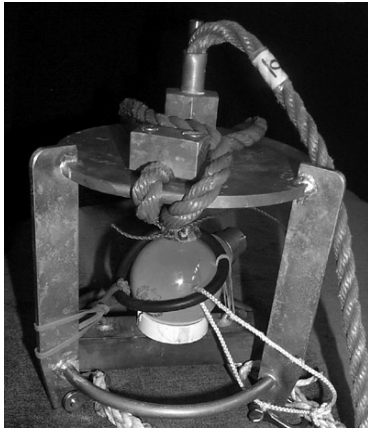
Figure 6 - Imploder device used to break light globes and evacuated spheres
