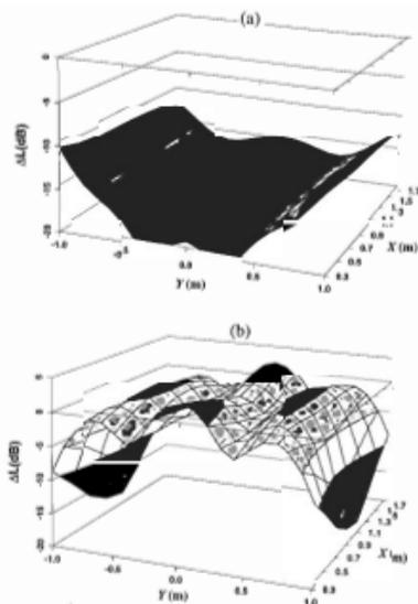
Figure 6. Extra sound attenuation due to the active noise control system when (a)  $r_{ss}=0.75\lambda$  and (b)  $r_{ss}=1.5\lambda$ .
