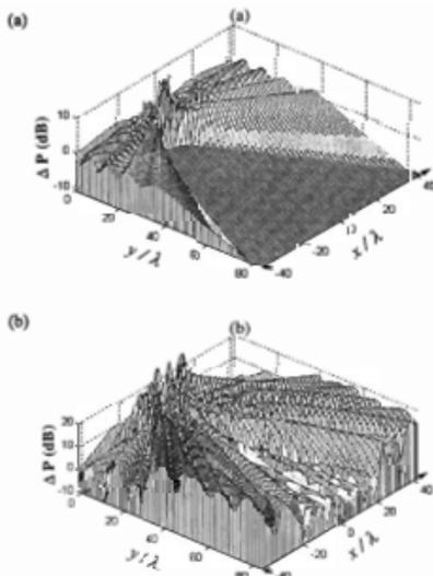
Figure 4. Sound pressure attenuation of a control system with 21 secondary sources and 21 error sensors when  $r_{ps}=5\lambda$ ,  $r_{es}=5\lambda$ , and (a)  $r_{sm}=0.715\lambda$ , and (b)  $r_{sm}=0.88\lambda$ .
