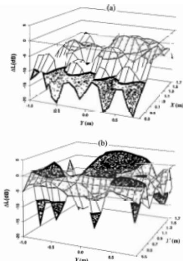
Figure 9. Extra attenuations due to the active noise control system when (a)  $r_{as}=0.75\lambda$  and (b)  $r_{as}=1.5\lambda$ .
