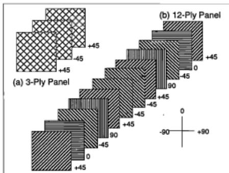
Figure 3. Lay-up of plies in 3-ply and 12-ply panels
