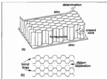
Figure 4. "Honeycomb Sandwich" panel, showing typical defects.
