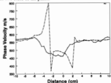
Figure 7. LPV scan across a delamination ----- on same face, ——— on opposite face of panel.
