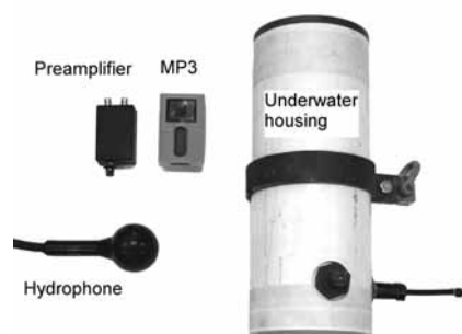
Figure 1. Components of the MP3 based underwater ambient noise recording system. The underwater housing is 16 cm in diameter and 42 cm in length.
